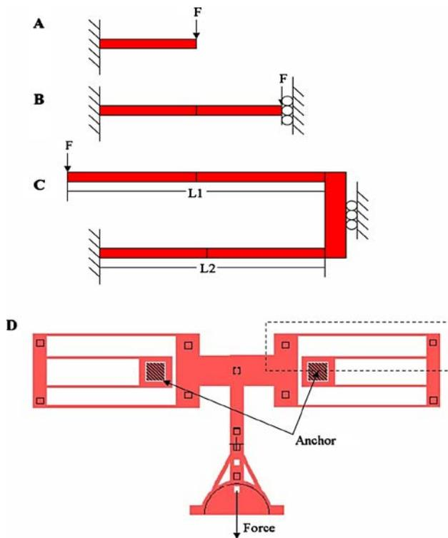
**Fig. 3** The spring constant of the folded-beam assembly is calculated by first taking a single cantilevered beam (A) and arraying it in series (B) with an identical beam. The free end of the folded-beam can be modeled as a roller support. These two beams are then in series with the beams fixed to the other end of the roller support (C). There are a total of four of these assemblies in parallel (indicated by the dashed box) for the entire spring
