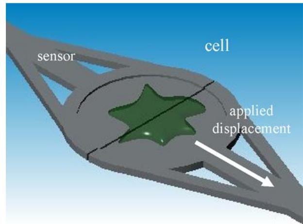
**Fig. 1** Basic concept of the cell tensometer
