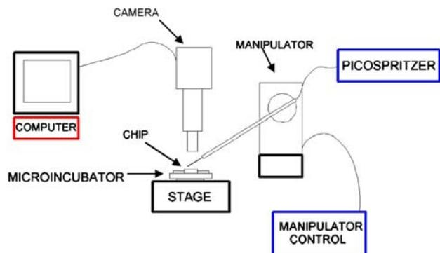
**Fig. 5** A probe station has been modified to accommodate all of the actuation, cell placement and imaging
