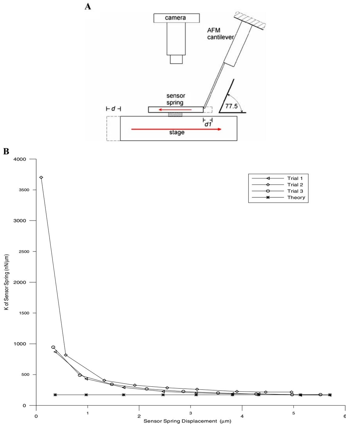
**Fig. 4** The calibration setup using a tipless AFM cantilever (A). The stage is moved relative to the stationary AFM tip a distance  $d$ , resulting in displacement  $d_1$  of the sensor spring. The stage is moved in one
