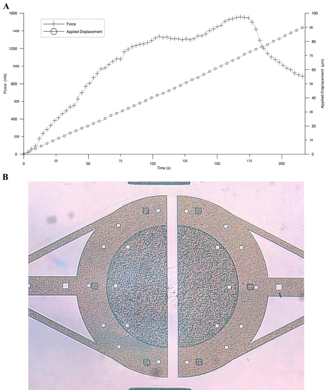
**Fig. 8** Force exerted on a fibroblast cell and the applied displacement as a function of time (A). Fibroblast cell being stretched during the experiment (B)
