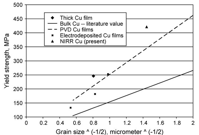
Fig. 3—A plot of yield strength against the reciprocal of the square root of the grain size (Hall-Petch plot). The material of the current study (NIRR for nanoindentation round robin) falls within the trend of other copper films, though it may be a little on the high side.
