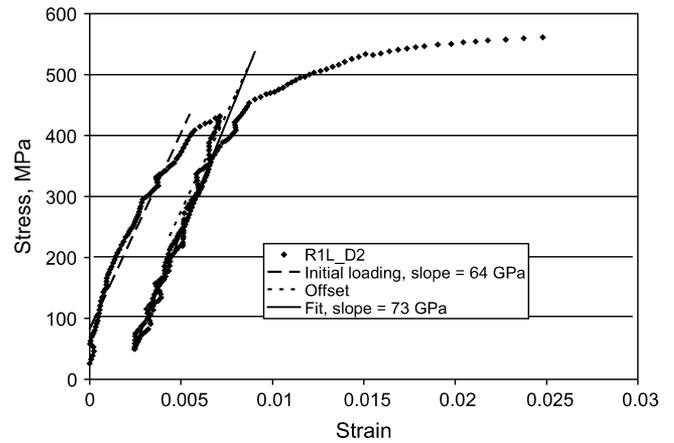
Fig. 2—Stress-strain curve for the Cu film of this study. The specimen was loaded, then unloaded to obtain a modulus value, and then loaded to failure.
