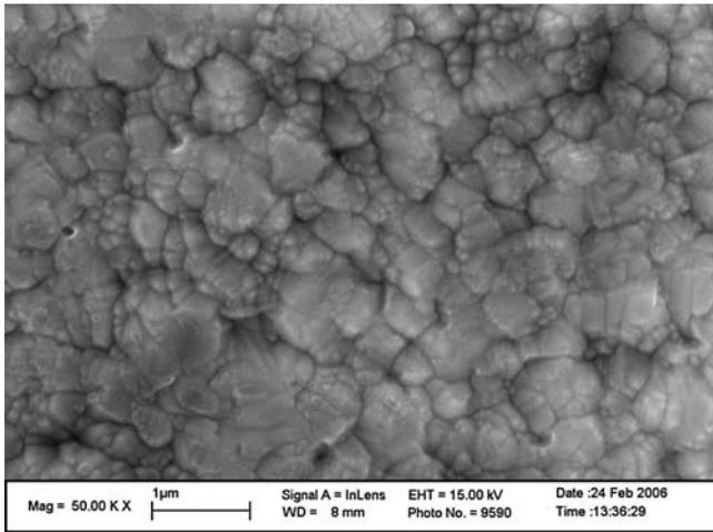
Fig. 1—SEM image of the surface of the Cu specimen film after preparation by ion milling. The imaging conditions are noted. The EBSD showed that the features correspond to crystallographic grains.
