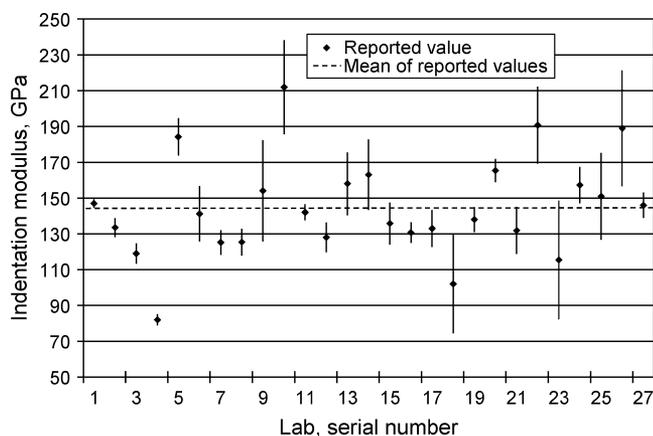
Fig. 5—Reported results for indentation modulus of the round robin specimen material, a Cu film on a silicon substrate. The error bars at each data point span a total range of 4 times the standard deviation reported for multiple indentations. The average of the reported modulus values is 144.5 GPa.
