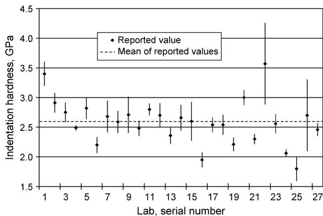
Fig. 4—Reported results for indentation hardness of the round robin specimen material, a Cu film on a silicon substrate. The error bars at each data point span a total range of four times the standard deviation reported for multiple indentations. The average of the reported hardness values is 2.59 GPa.
