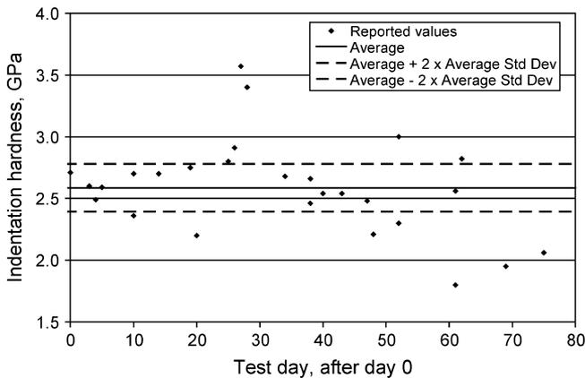
Fig. 8—Reported indentation hardness values plotted against test day, counted from an arbitrarily selected day 0. The data plotted here show that there are no statistically significant effects of specimen aging.
