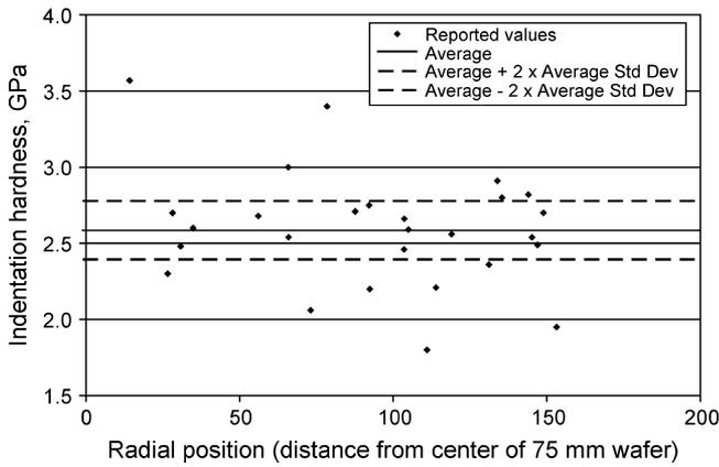
Fig. 7—Indentation hardness plotted against radial position of the respective specimen chip. These data show that there is no statistically significant effect of the location of the chip on the measured indentation hardness.
