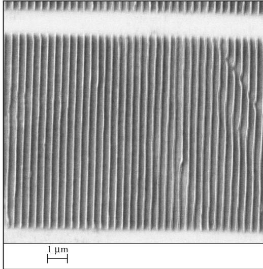
**Figure 1.** SEM image of a section of the array of PMMA nanolines.
