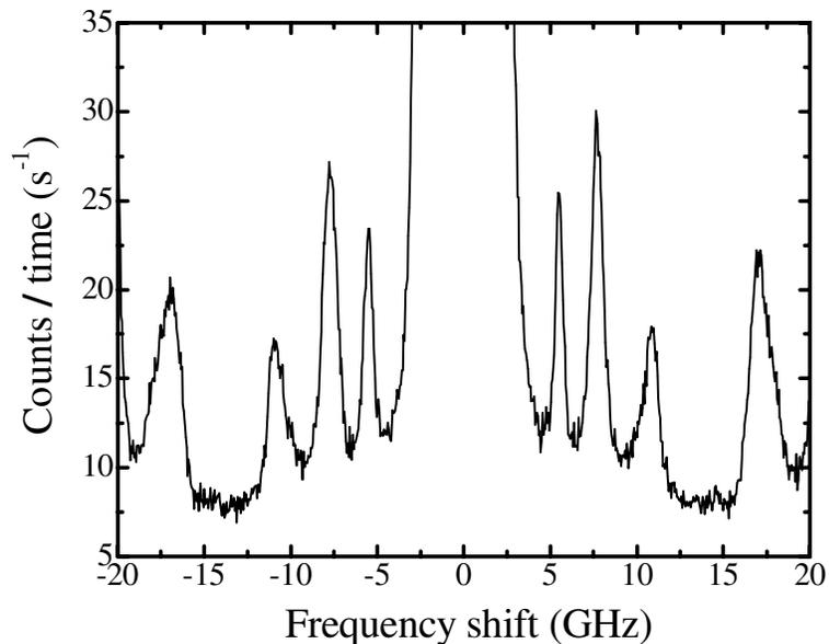
**Figure 2.** BLS spectrum with an angle of  $70^\circ$  between the substrate normal and the incident beam. Ordinates are the counts per unit time in one channel of the multichannel analyzer.
