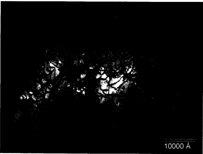
FIGURE 4.8. TEM micrograph of a thin film of microtensile specimen of aluminum, strained to failure in tension. The dark lines are dislocations. The dislocation density is about 10^{11} \text{ cm}^{-2} .
