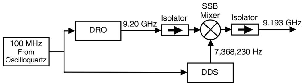
**Figure 4.** A schematic layout of the most recent microwave synthesizer developed for NIST-F1. A 100 MHz reference signal is fed to a DRO module that multiplies by 92 up to 9.20 GHz. This is mixed with an RF signal at 7.368 23 MHz from a DDS unit, also referenced to the 100 MHz, in an SSB mixer to produce microwaves at the Cs clock transition.
