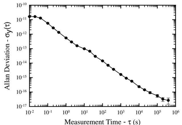
**Figure 3.** An Allan deviation plot of the two 5 MHz signals fed into the time-difference analyser in the microwave monitoring system illustrating that the microwave synthesizer is a negligible noise source in NIST-F1. The y-axis has been scaled to show the fractional frequency stability referenced to the 9 GHz sources. The stability at  $\sim 4 \times 10^5$  s is below  $3 \times 10^{-17}$ .
