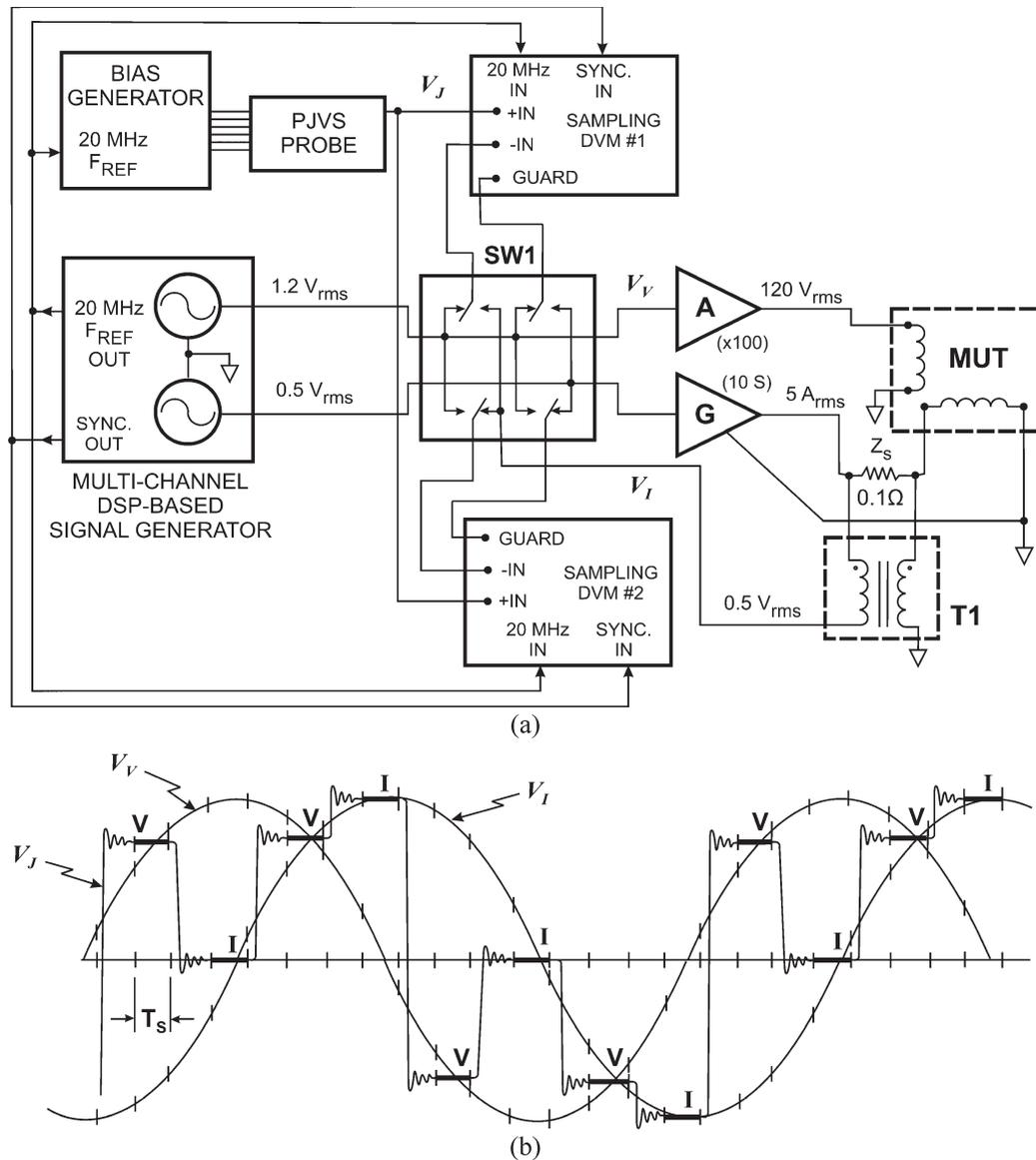
Fig. 1. Quantum-based power generation system. (a) Simplified diagram, including sampling DVMs operating in the differential voltage sampling mode. (b) How a single PJVS waveform  $V_J$  is used to provide reference levels for the differential sampling of the two scaled voltages  $V_V$  and  $V_I$ . The bold intervals of  $V_J$  represent the sampling intervals of interest; the remaining sampling intervals are ignored.
