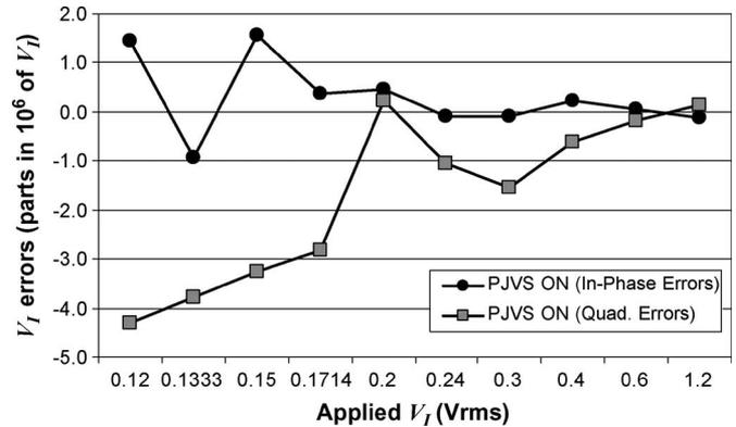
Fig. 3. PJVS-derived  $V_V/V_I$  ratio accuracy tests measured using a permuting capacitance divider. The  $V_V$  signal was set to 1.2 V RMS (DVM range = 100 mV).
