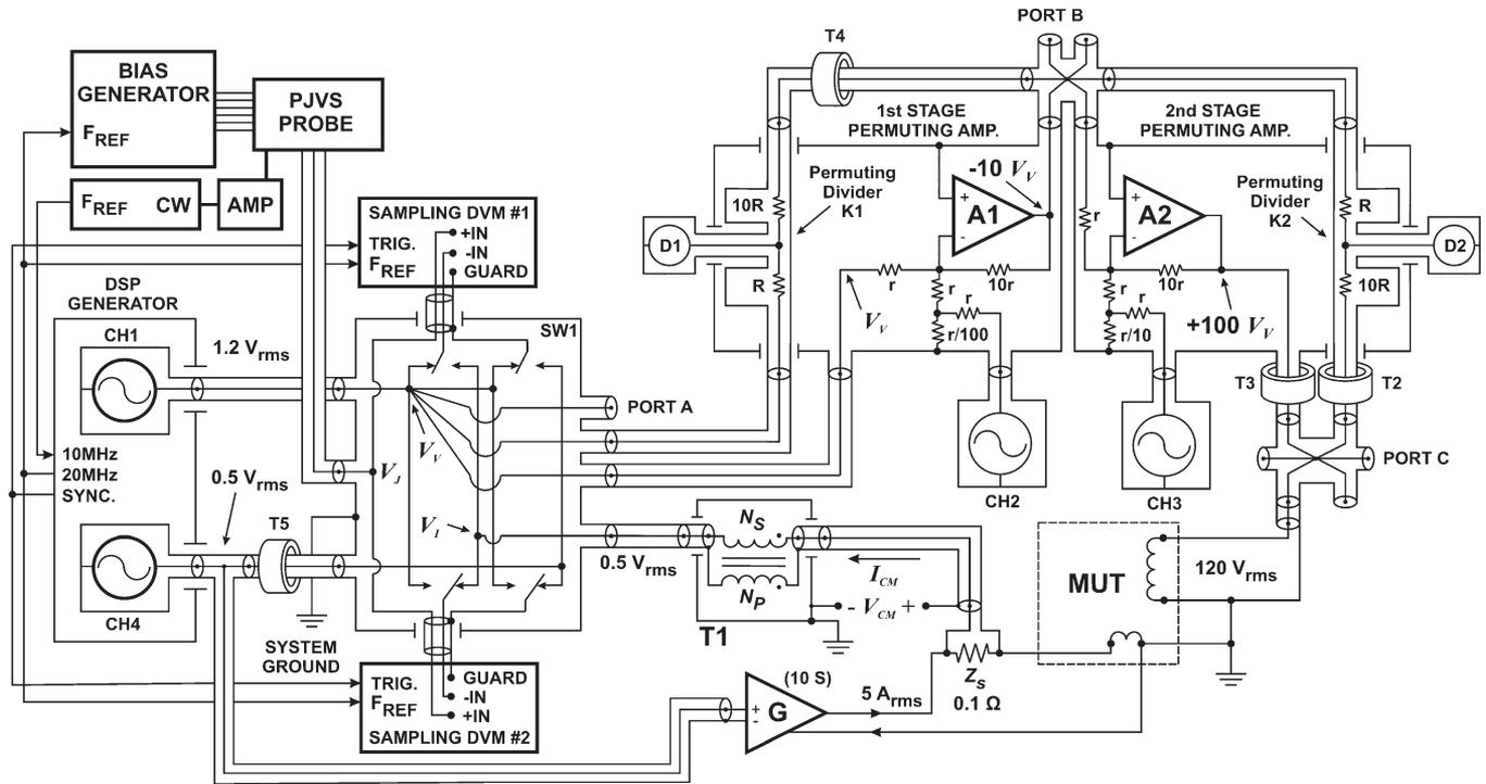
Fig. 5. Detailed diagram of the quantum-based power generation system detailing the permuting amplifier design and component interconnection requirements.
