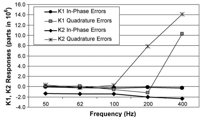
Fig. 6. K1 and K2 permuting divider responses as measured against a permuting capacitance reference divider.
