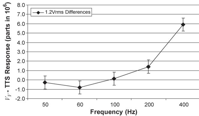
Fig. 2. Measured differences between the 1.2 V RMS PJVS-derived  $V_V$  signal and a calibrated TTS.
