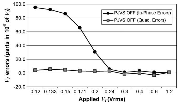
Fig. 4. Non-PJVS-derived  $V_V/V_I$  ratio accuracy tests measured using a permuting capacitance divider. The  $V_V$  signal was set to 1.2 V RMS (DVM range = 10 V).
