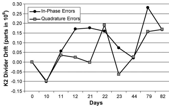
Fig. 7. Stability analysis of the K2 divider errors versus a permuting capacitance divider.
