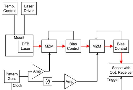
Fig. 1. Block diagram of cascaded modulator setup.
