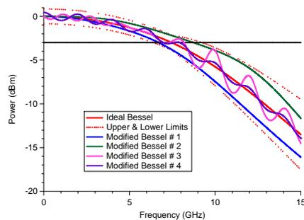
Fig. 3. Frequency response of non-ideal filters.
