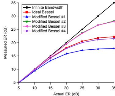
Fig. 4. Simulated ERs for non-ideal filters.
