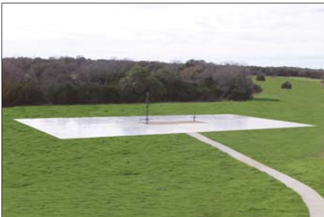
Figure 2: An example of an Open Area Test Site (OATS) used for calibrating antennas (photo courtesy of ETS-Lindgren)
