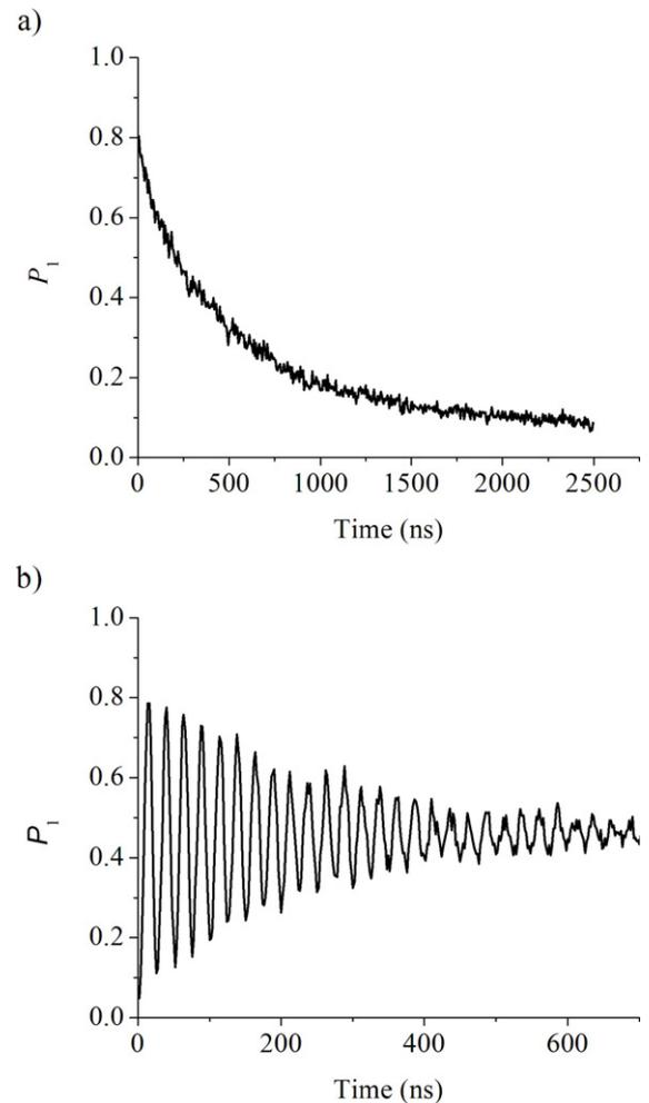
**Figure 3.** Low-temperature ( $T = 20$  mK) measurements for the qubit with a c- $\text{Al}_2\text{O}_3$  tunnel barrier. (a) Energy relaxation time  $T_1 = 500$  ns. Measurement fidelity = 80%. (b) Rabi oscillations: dephasing time  $T_2 \sim 140$  ns. Rabi visibility = 70%.
