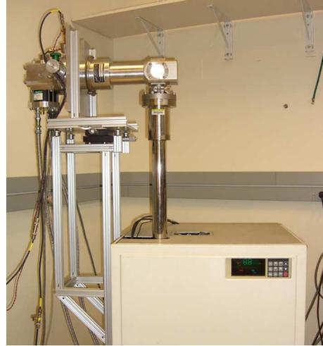
Fig. 3. Photographs of the integrated system with the cryostat bolted onto the MALDI-TOF mass spectrometer.
