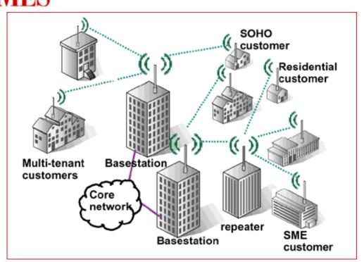
With the completion of the IEEE Standard 802.16(r) WirelessMAN air interface, broadband wireless access (BWA) is reaching maturity as an alternative for broadband access deployment. Once the 802.16a amendment is complete, the standard will specify interoperable wireless metropolitan area network (wireless MAN) air interfaces from 2-66 GHz, including licensed and license-exempt operation, under a single umbrella with a common medium access control layer (MAC). Source: Nokia Networks
