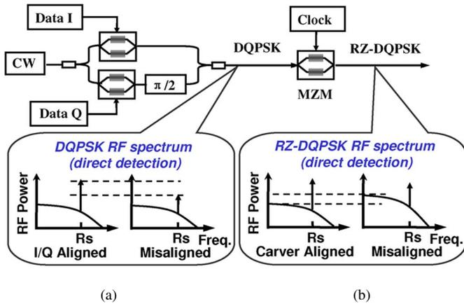
Fig. 1. Conceptual diagram of misalignment monitoring for RZ-DQPSK transmitters. (a) Misalignment between I/Q data. Clock tone power at symbol rate decreases with I/Q misalignment. RF power at low frequencies increases with carver/data misalignment. (b) Misalignment between carver and data. RF power at low frequencies increases with carver/data misalignment.
