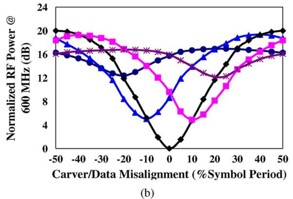
Fig. 3. Simulated RF power versus time misalignment. (a) I/Q data misalignment; (b) carver/data misalignment with and without I/Q data misalignment.
