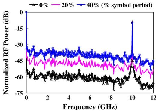
Fig. 2. Simulated RF spectra in the presence of carver/data misalignment.
