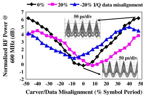
Fig. 6. Measured low-frequency power versus carver/data misalignment.
