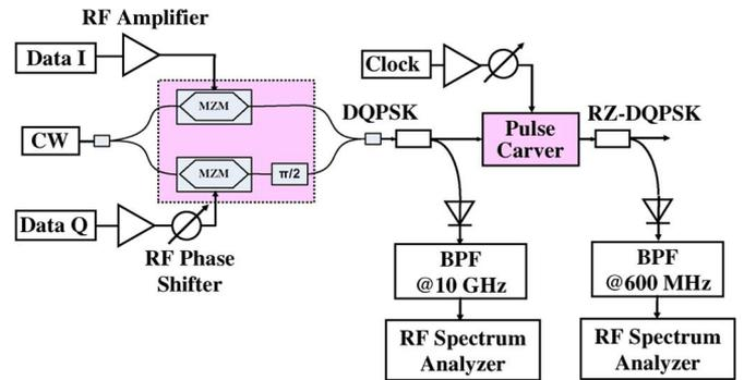
Fig. 4. Experimental setup for RZ-DQPSK misalignment monitoring.
