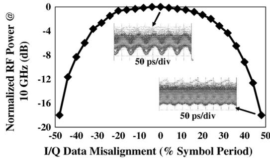
Fig. 5. Measured clock tone power of the 20-Gb/s DQPSK signal versus I/Q data misalignment. Clock tone power decreases with the misalignment.
