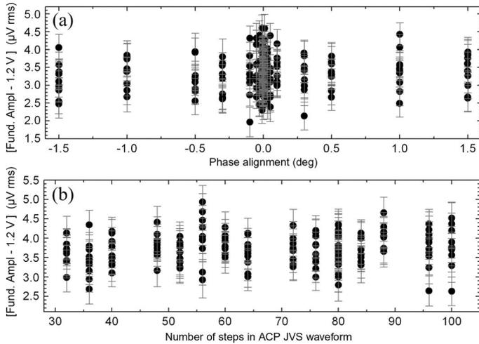
Fig. 5. Demonstration that the differential sampling method produces consistent results with regard to (a) phase misalignment and (b) number of steps in the ACPJVS waveform.
