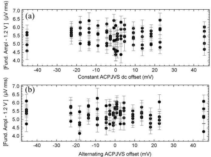
Fig. 6. Demonstration that the differential sampling method produces consistent results with regard to (a) ACPJVS dc offsets and (b) ACPJVS interleaved offsets.
