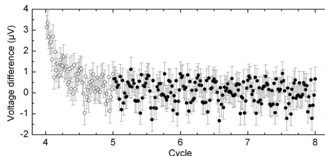
Fig. 8. Difference between the expected Josephson rms voltage (10 mV) and the amplitude measured with the sampling voltmeter as a function of time (50 Hz cycle). During cycles 1 through 4, the 100 mV range of the sampling voltmeter is overloaded with the 1.2 V juxtaposed waveform. After a complete cycle (open circles), the sampler fully recovers from the overloaded state (solid circles).
