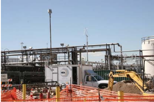
Figure 2: The receiver was located inside a van with antennas top-mounted on a mast approximately 7.5 m (25 feet) above the ground.
