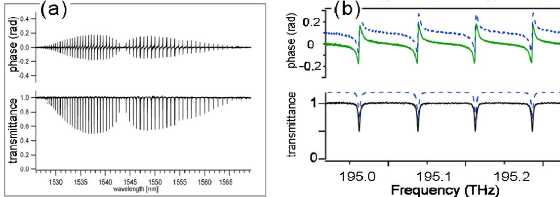
**Figure 2(a)** Measured phase and absorption spectrum for hydrogen cyanide (HCN). In total the measurement spanned from 1492 nm to 1618 nm or 155,000 individual frequency comb lines. For clarity only the data showing HCN absorption bands is shown. (b) Expanded view, data is in excellent agreement with previously published values [8] (dotted lines offset for clarity).
