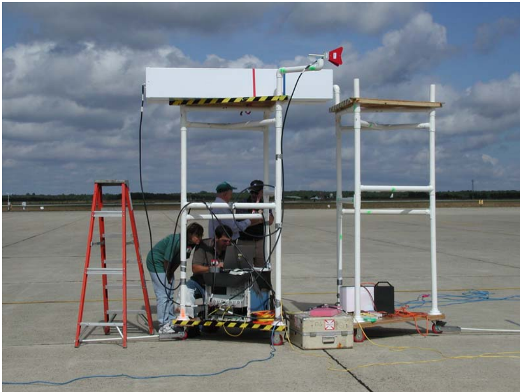
Figure 6. Reference measurement setup. The transmitting tower is configured and the receiving antennas will be mounted on top of the second tower.
