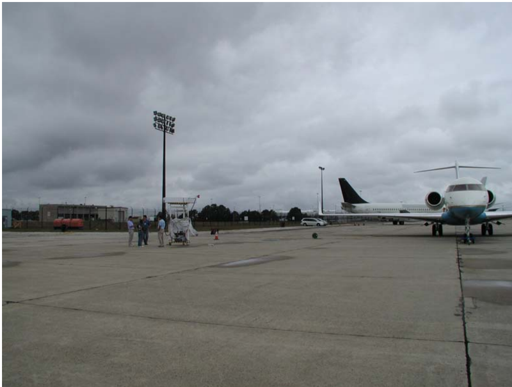
Figure 7. The transmitting antennas placed on top of a support tower and boresighted at the center of the aircraft.
