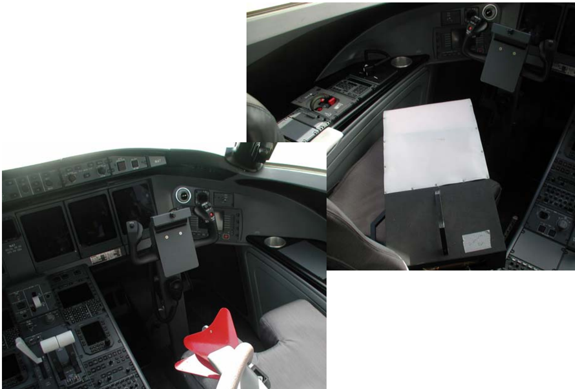
Figure 54. The receiving DRG and TEM antennas placed between the pilot and co-pilot seat as shown in these two photos.
