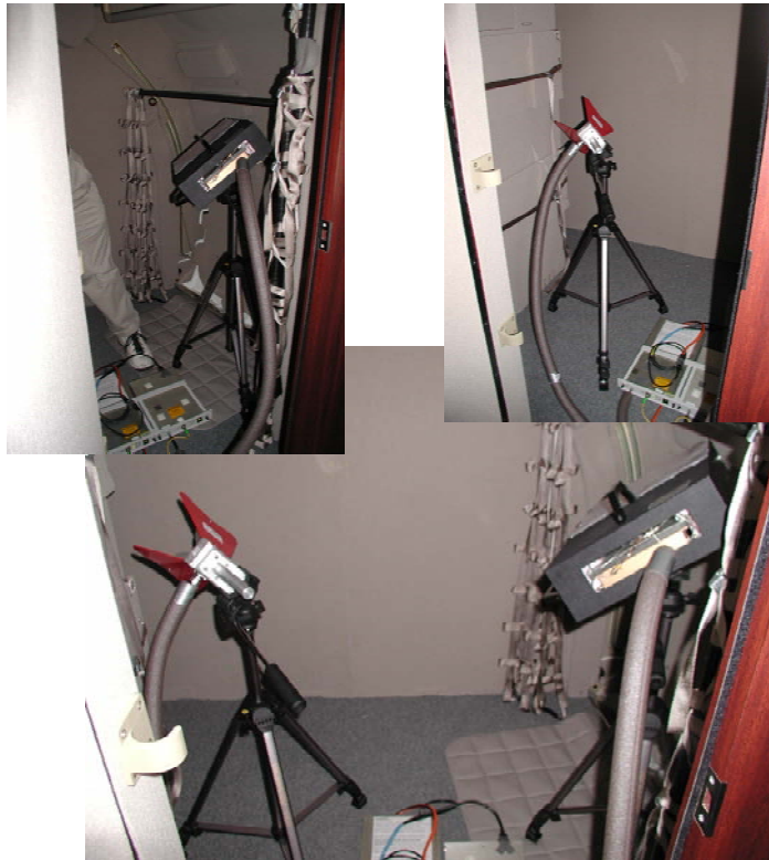
Figure 87. TEM and DRG antenna placement in the cargo closet.
