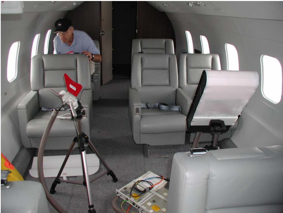
Figure 19. Receiving antenna placement in main passenger cabin.
