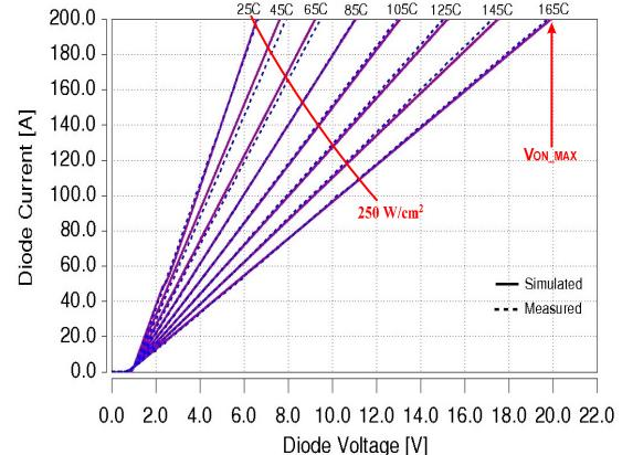
**Fig. 3:** Comparison of scaled measured (dashed) and simulated (solid) forward conduction characteristics at 25 °C, 45 °C, 65 °C, 85 °C, 105 °C, 125 °C, 145 °C, and 165 °C for a 100 A, 10 kV SiC JBS diode.
