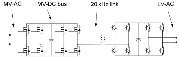
**Fig. 8:** Example of a building block circuit for an SSPS. This building block converts medium voltage AC (MV-AC) at the primary (PRI) to low voltage AC (LV-AC) at the secondary (SEC).
