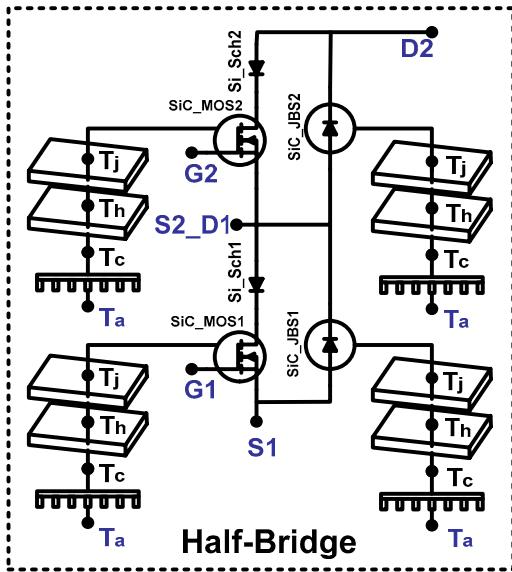
**Fig. 5:** Circuit topology of the half-bridge SiC MOSFET/JBS power module with low-voltage series diodes to prevent reverse conduction in the MOSFETs. The thermal network component models representing heat transport within the module are also indicated.
