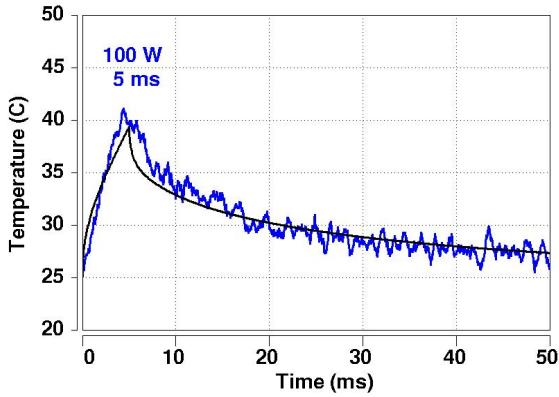
**Fig. 6:** Measured (blue) versus simulated (black) SiC MOSFET junction temperature for a 100 W, 5 ms chip dissipated power pulse ( $A_{\text{MOSFET}} = 0.1545 \text{ cm}^2$ ).
