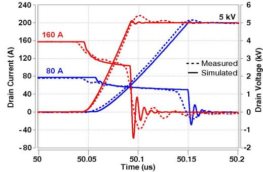
**Fig. 2:** Comparison of scaled measured (dashed) and simulated (solid) inductive-load switching turn-off waveforms at 25 °C for a clamp voltage of 5 kV and a 100 A, 10 kV SiC power MOSFET.
