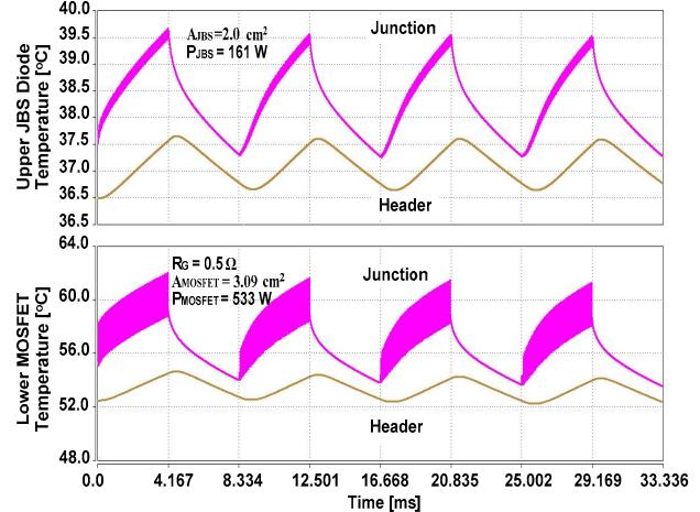
**Fig. 7:** Temperature waveforms for lower SiC MOSFET with  $R_G=0.5 \Omega$  and  $A_{\text{MOSFET}} = 3.09 \text{ cm}^2$  and the upper SiC JBS diode with  $A_{\text{JBS}} = 2.0 \text{ cm}^2$  in the 100 A, 10 kV half-bridge power module.
