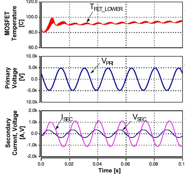
**Fig. 9:** Simulated waveforms for the circuit of Fig. 8 with an optimized module configuration similar to Case 5 of Table 1.
