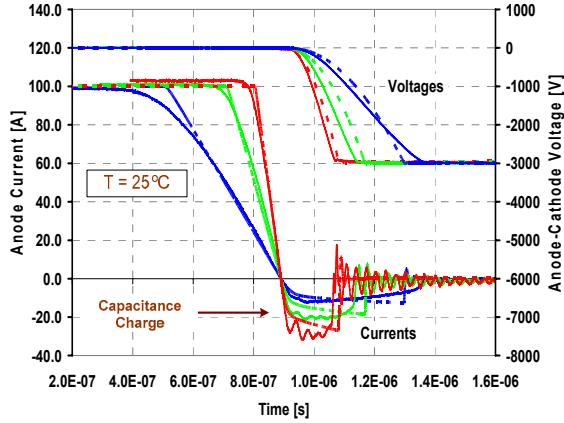
**Fig. 4:** Comparison of scaled measured (solid) and simulated (dashed) reverse recovery characteristics at  $25^\circ\text{C}$  for a 100 A, 10 kV SiC JBS diode.
