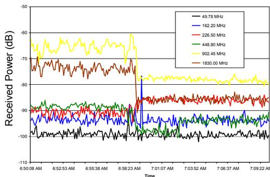
Figure 2: Received power verses time during the collapse of the: (a) apartment building and (b) sports stadium.
