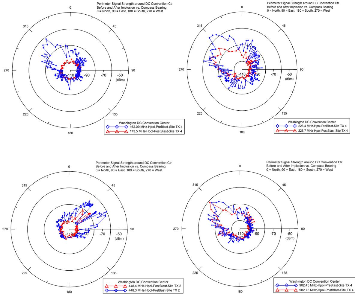
Figure 3: Comparison of pre- and post-implosion received signal level, as measured with the mobile cart for the convention center.
