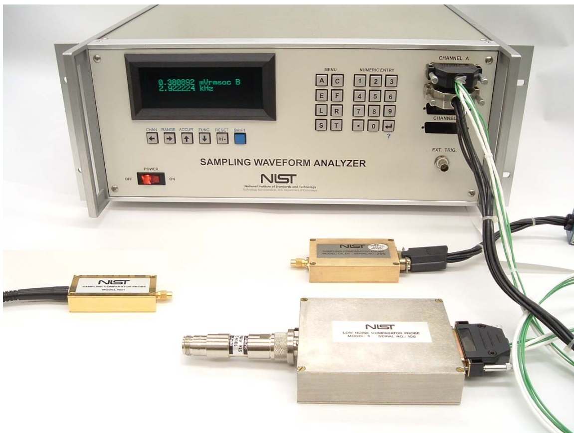
Fig. 3. Picture of SWA system showing mainframe unit, low-noise sampling probe with 100 V attenuator attached (foreground), ASIC sampling probe (nearest to mainframe), and the Next Generation Sampling Comparator Probe (left).
