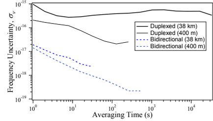
Fig. 1c. Allan deviation for duplexed and bidirectional fiber configurations of 38 km (installed) and 400 m (spooled).
