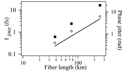
Fig. 2b. Integrated jitter: total timing jitter (squares), jitter without servo bump contribution (circles), theoretical prediction from integrating  $S_{Locked}$  (line).
