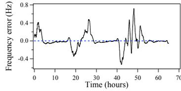
Fig. 1b. Counted frequency error (difference from transmitted frequency) for 38 km link in bidirectional (dashed) and duplexed (solid) configuration.
