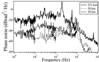
Fig. 2a. Phase noise spectra of locked one-way transmission at various link lengths.
