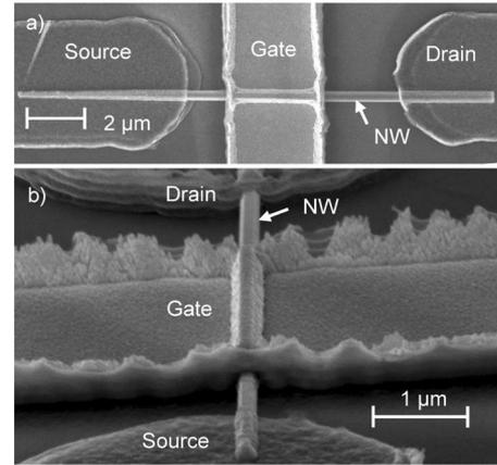
Fig. 2. (a) FESEM image of a typical NW MESFET as seen from the top. (b) FESEM image of an NW MESFET as seen from an angle looking down the length of the NW, showing the omega gate structure. The flagging metal edges are due to the lift-off process.
