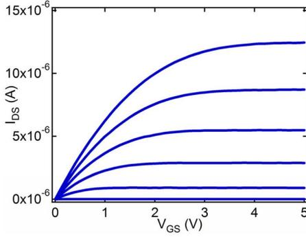
Fig. 5. Drain–source current ( $I_{DS}$ ) versus drain–source voltage ( $V_{DS}$ ) at several gate–source voltages ( $V_{GS}$ ) showing the best example of saturation observed for a single-NW MESFET. The bottommost trace corresponds to  $V_{GS} = -3$  V, with  $\Delta V_{GS} = 0.5$  V between successive traces proceeding upward.
