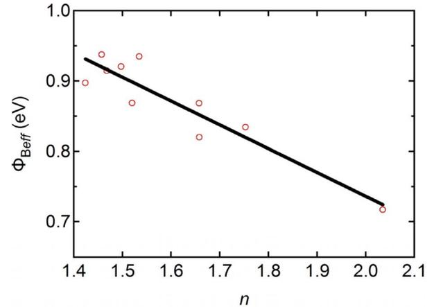
Fig. 4. Estimated values of effective Schottky barrier height ( $\Phi_{B,\text{eff}}$ ) versus ideality factor ( $n$ ) with linear fit for ten devices. The equation of the linear fit is  $\Phi_{B,\text{eff}} = -0.34n + 1.41$  eV. From the fit, the homogeneous Schottky barrier height  $\Phi_{B_0}$  was estimated to be approximately 1.1 eV.
