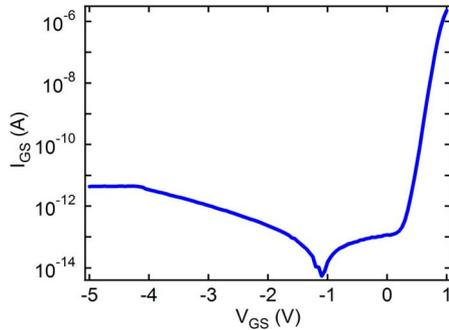
Fig. 3. Log-linear plot of the magnitude of gate-source current ( $I_{GS}$ ) versus gate-source voltage ( $V_{GS}$ ) for a typical device. The minimum at  $V_{GS} \approx -1.2$  V is where  $I_{GS}$  crosses from positive to negative. However, it is suspected that noise contributes strongly to the measurement when the magnitude of  $I_{GS}$  is less than approximately 100 fA ( $10^{-13}$  A).
