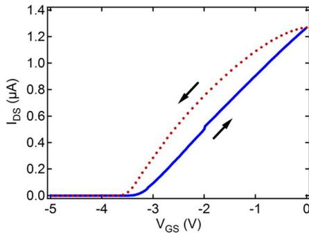
Fig. 7. Hysteresis in drain-source current ( $I_{DS}$ ) versus gate-source voltage ( $V_{GS}$ ) at drain-source voltage ( $V_{DS}$ ) of 0.1 V for a single-NW MESFET.  $V_{GS}$  was swept from  $-5$  to  $0$  V (solid trace), and then immediately swept from  $0$  to  $-5$  V (dotted trace). The maximum offset between the two sweeps is approximately 600 mV.
