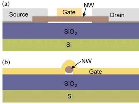
Fig. 1. (a) Schematic cross section of NW MESFET structure as seen from the side. The gap between the NW and the  $\text{SiO}_2$  is exaggerated for clarity; in fabricated devices, the NW is effectively in contact with the  $\text{SiO}_2$ . (b) Schematic cross section of NW MESFET as seen looking down the axis of the NW, showing the omega gate structure. From FESEM inspection, the omega gate is estimated to cover one-half to two-thirds of the NW circumference.
