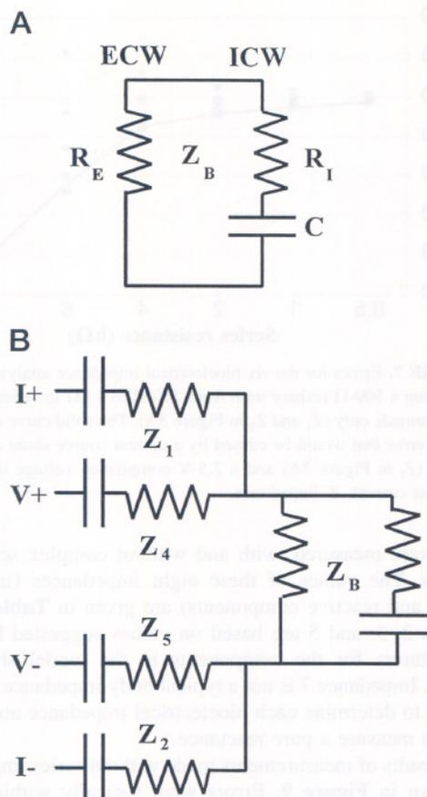
**FIGURE 4.** A) The commonly used extracellular water (ECW)–intracellular water (ICW) model of the deep body tissue.  $R_E$ , extracellular resistance;  $Z_B$ , deep-tissue impedance;  $R_I$ , intracellular resistance;  $C$ , cell membranes. B) The whole-body model, including the ECW-ICW model with simulated surface impedances added (plus and minus signs are used only to identify the two different sets of leads, not to indicate polarity).  $I$ , current;  $V$ , voltage.
