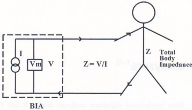
**FIGURE 1.** Two-terminal body impedance measurement method. *I*, current; *V<sub>m</sub>*, voltmeter; *V*, voltage; BIA, bioelectrical impedance analyzer; *Z*, impedance.
