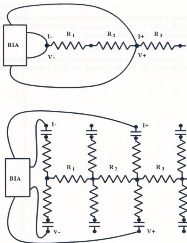
**FIGURE A1.** User tests to evaluate bioelectrical impedance analyzers for a particular task. The top part of the figure is a test to measure the dynamic range of an analyzer; the bottom part of the figure is a test to simulate surface impedance.
