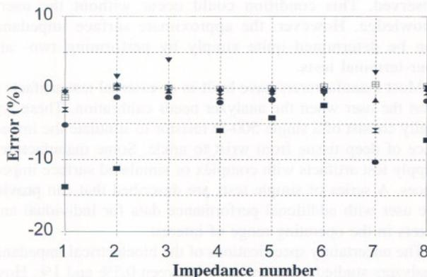
FIGURE 9. Errors for the six bioelectrical impedance analyzers tested in measuring eight complex impedances, which were selected to simulate a range of deep-tissue impedances without simulated surface impedance (Figure 4A).
