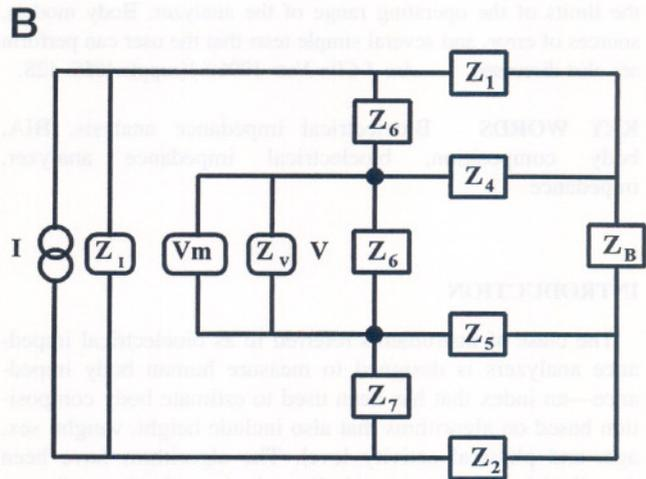
**FIGURE 3.** A) Block diagram model of the impedances encountered in a measurement of deep-body impedance. *I*, current; *Z*, impedance; *Z<sub>1</sub>*, current impedance; *V<sub>m</sub>*, voltmeter; *Z<sub>S</sub>*, voltmeter impedance; *V*, voltage; *Z<sub>B</sub>*, deep-body impedance. B) The circuit diagram used to simulate the interaction of various impedance components.
