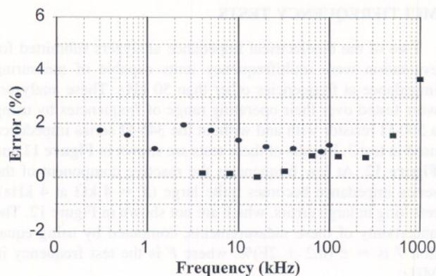
FIGURE 11. Error versus frequency of two multifrequency bioelectrical impedance analyzers measuring a 500- $\Omega$  resistor without simulated surface impedance.
