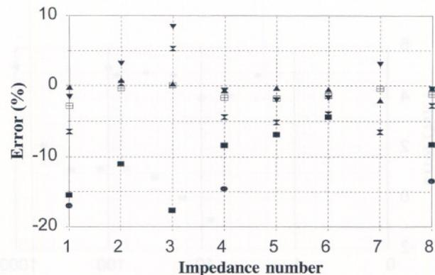
FIGURE 10. Errors in the six bioelectrical impedance analyzers tested in measuring the same eight complex impedances as in Figure 9, but with a 345- $\Omega$  simulated surface impedance in series with each terminal (see Figure 4B).
