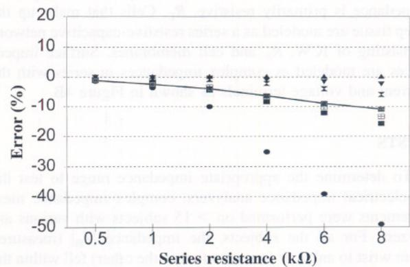
**FIGURE 8.** Errors for the six bioelectrical impedance analyzers tested in measuring a 500- $\Omega$  resistor with from 250  $\Omega$  to 4 k $\Omega$  in series with the voltage terminals only ( $Z_4$  and  $Z_5$  in **Figure 3A**). The solid curve shows the simulated error that would be caused by a voltmeter shunt resistance of 64 k $\Omega$  ( $Z_V$  in **Figure 3A**).  $Z$ , impedance.
