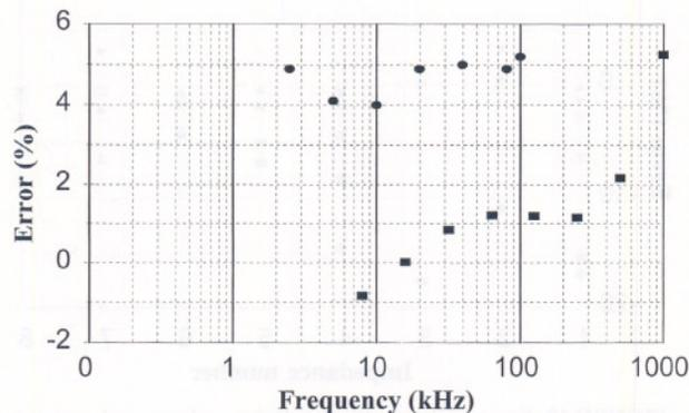
FIGURE 12. Error versus frequency of two multifrequency bioelectrical impedance analyzers measuring a 500- $\Omega$  resistor with a 345- $\Omega$  simulated surface impedance in series with each terminal.
