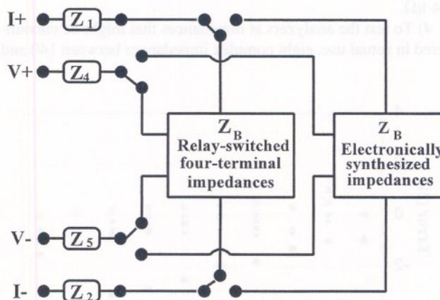
**FIGURE 5.** Block diagram of the impedance generator used in the bioelectrical impedance analyzer evaluation.  $Z_B$  (deep-tissue impedance) is simulated by relay-switched components (resistors and capacitors) or by electronically synthesized signals applied to the analyzer's voltage terminals. Simulated surface impedances can be placed in series with any of the terminals.  $I$ , current;  $Z$ , impedance;  $V$ , voltage.
