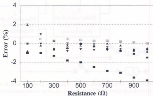
**FIGURE 6.** Errors for the six bioelectrical impedance analyzers tested as basic alternating-current resistance meters from 100 to 1000  $\Omega$  without series resistance.
