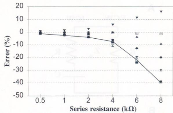
**FIGURE 7.** Errors for the six bioelectrical impedance analyzers tested in measuring a 500- $\Omega$  resistor with from 250  $\Omega$  to 4 k $\Omega$  in series with the current terminals only ( $Z_1$  and  $Z_2$  in **Figure 3A**). The solid curve shows the simulated error that would be caused by a current source shunt resistance of 64 k $\Omega$  ( $Z_1$  in **Figure 3A**) and a 2.5-V compliance voltage limit for a 0.5-mA test current.  $Z$ , impedance.
