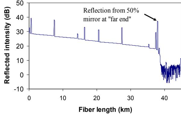
**Fig. 2** Optical Time Domain Reflectometry (OTDR) trace for the 38 km long BRAN fiber: end-to-end loss 8.3 dB (0.2 dB/km). Reflected intensity spikes indicate locations where the fiber comes above ground to a patch panel.
