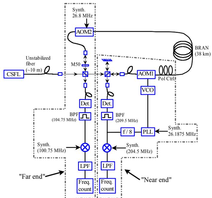
**Fig. 1** Experimental setup. AOM, acousto-optic modulator; BPF, bandpass filter; BRAN, 38 km installed fiber loop; CSFL, cavity-stabilized fiber laser; Det., detector;  $f/8$ , 8x frequency divider; LPF, low-pass filter; M50, 50 % reflecting mirror; PLL, phase-lock loop; Synth., frequency synthesizer; VCO, voltage-controlled oscillator.
