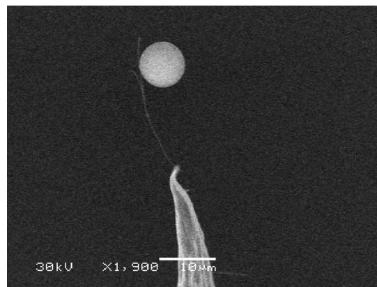
Fig. 4 A micrograph of a typical sphere-nanotube structure that we constructed, consisting of an 8- \mu\text{m} sphere suspended by a \sim 100-nm-diam multiwall carbon nanotube. The novel structure was used to compare measured scattering spectra to Mie theory calculations.
