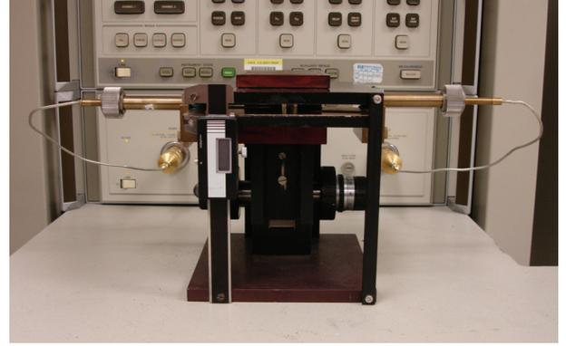
FIGURE 2: A parallel-plate resonator measurement fixture.
