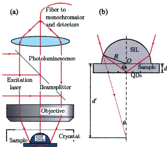
FIG. 1. (Color) The optical setup of the experiment. (a) Overview of optical layout. NAIL-sample assembly is placed inside a microscopic cryostat, which moves in  $X$  and  $Y$  directions during a 2D scan. (b) Optics of the NAIL-sample assembly. The hemispherical SIL is placed on the back side of the sample, whose thickness  $d$  satisfies  $d=R/n$  for stigmatic imaging.
