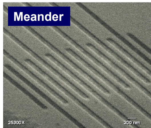
Fig. 3. Scanning electron microscope image of an SSPD meander device similar to the one discussed in the text.
