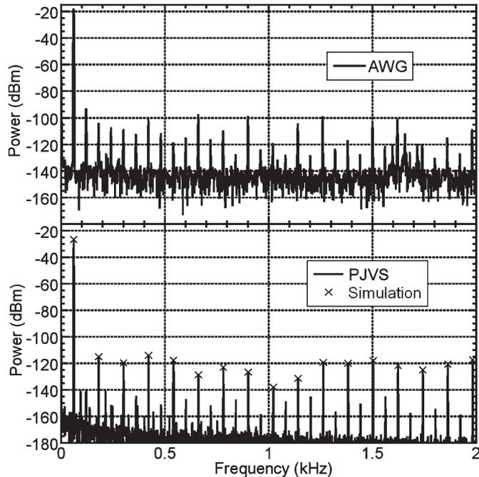
Fig. 3. Spectral content of a 512 sample sinewave at 60 Hz generated by a Josephson array with 2.1 V amplitude zero-to-peak ( $1.5 V_{\text{rms}}$ ). The PJVS measured spectrum (black, lower plot) shows excellent agreement with numerical simulations (gray). The upper plot shows the spectrum from a semiconductor AWG measured with the same digitizer and plotted on the same scale.
