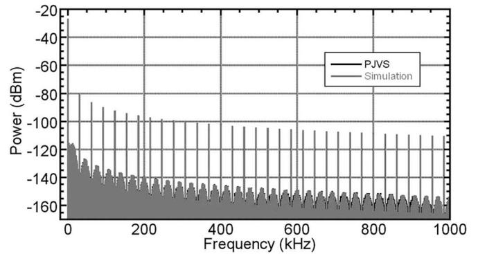
Fig. 2. Spectral measurement of a 512 sample 60 Hz sinewave generated by a Josephson array with 2.1 V amplitude zero-to-peak ( $1.5 V_{rms}$ ). Measured harmonics from the Josephson array (black) is in excellent agreement with the numerical simulations (the gray simulation curve exactly covers the black measured data).
