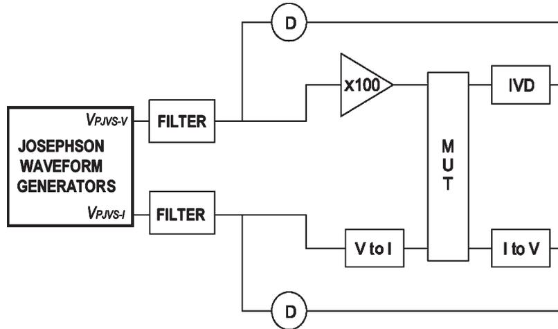
Fig. 1. Schematic of one possible implementation of the power standard with two Josephson reference voltage waveforms and other essential components. The symbol “D” denotes high-precision phase-sensitive detectors.
