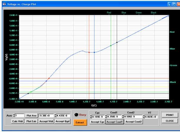
**Fig. 4b:** Voltage vs. charge plot sub-panel demonstrating the extraction of  $C_{GS}$ ,  $C_{OXD}$ ,  $V_T$ , and  $V_{TD}$ .
