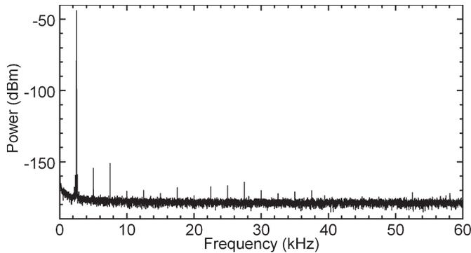
Fig. 5. Digitally sampled spectral measurement of a 200 mV sine wave at 2.5 kHz synthesized by use of new ACJVS circuits with twice the number of junctions. These observed distortion harmonics are attributed primarily to inaccurate ACJVS operation.
