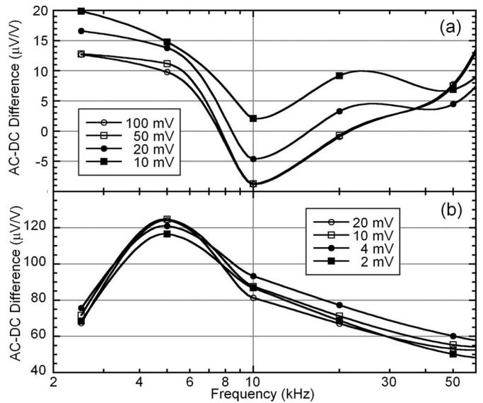
Fig. 3. AC–DC differences versus the frequency for the different rms voltages (2 mV to 100 mV) on the (a) 220 mV and (b) 22 mV ranges of the transfer standard, derived from ACJVS-synthesized waveforms. Connecting lines are merely guides to the eye.
