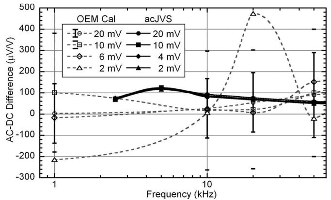
Fig. 4. AC–DC differences versus the frequency on the 22 mV range of the transfer standard with rms amplitudes ranging from 2 mV to 20 mV. Solid symbols denote ACJVS measurements. Open symbols denote the manufacturer’s specified calibration, with error bars (20 mV) or error “caps” (10 mV) shown for the two largest voltages. Connecting lines are merely guides to the eye.
