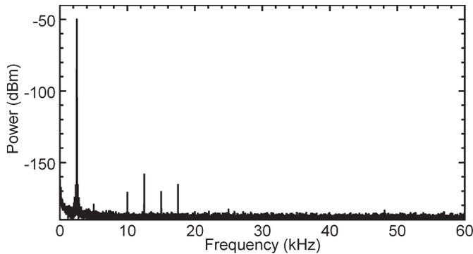
Fig. 1. Digitally sampled spectral measurement showing harmonic distortion tones at  $-110$  dBc [in decibels below the fundamental (carrier)] for the 2 V range of the digitizer and attributed to digitizer nonlinearities. Both Josephson arrays are used to generate the 100 mV (rms) sine wave at 2.5 kHz. The digitizer used  $1\text{ M}\Omega$  input impedance, 10 Hz resolution bandwidth, ten averages, and 1 MS/s sampling rate.
