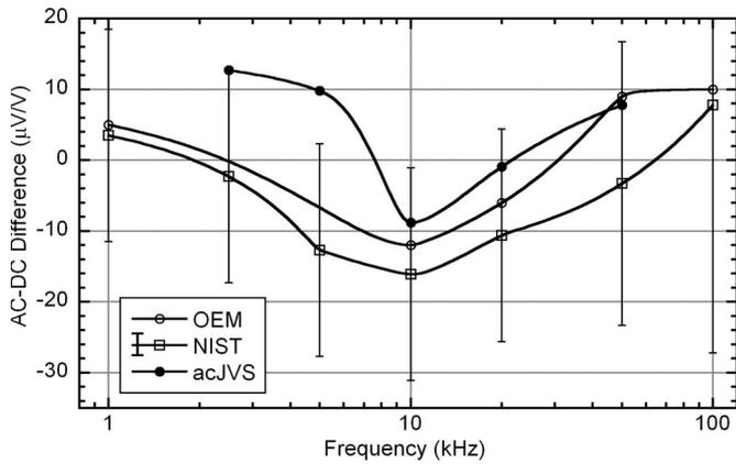
Fig. 2. AC–DC differences versus frequency for 100 mV rms signals measured on the 220 mV range of the transfer standard, comparing the manufacturer (OEM) and NIST calibrations (open symbols) with the corrected ACJVS measurements (solid symbols). Error bars show the NIST calibration uncertainty.
