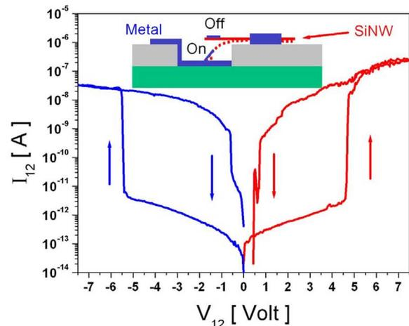
Fig. 8. (a) SEM image of SiNW NEMS (Scale bar: 10  $\mu$ m). Suspended gap is 400 nm. SiNW is about 150 nm in diameter. (b) Plot of switching current ( $I_{12}$ ) as a function of switching voltage ( $V_{12}$ ). Inset of (b) shows schematic of NEMS switch ON/OFF as the SiNW is bent by electrostatic force.
