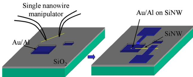
Fig. 7. Schematics of fabrication of nanoelectromechanical switch with SiNW suspended above a metal pad by using method I.
