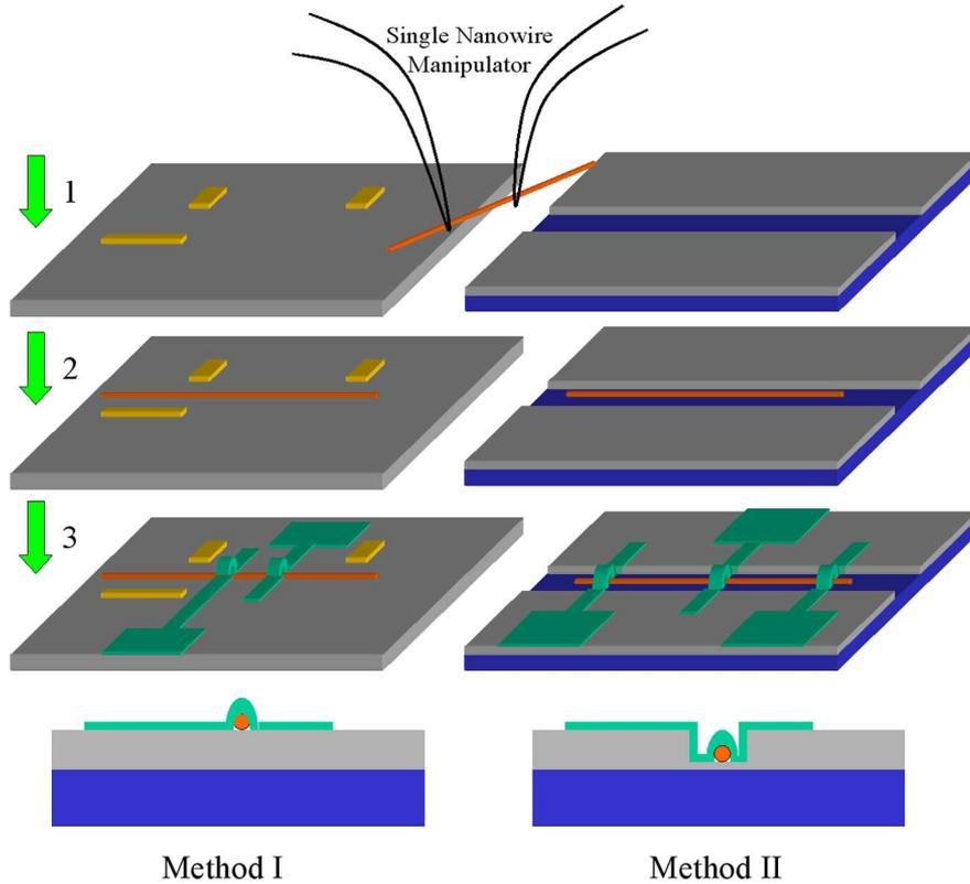
Fig. 3. Two methods (I on the left side and II on the right side) used to align the nanowires. Step 1: placing a single nanowire on a flat (method I) or trench (method II) substrate. Step 2: precision alignment of the nanowire with the substrates. Step 3: formation of metal contacts.
