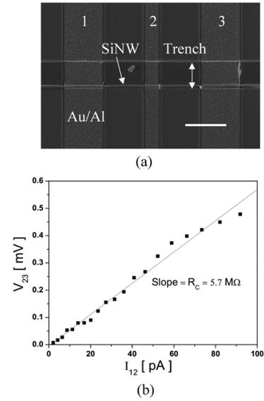
Fig. 5. (a) SEM image of Kelvin test structure for characterization of metal/SiNW contact resistance (Scale bar: 5  $\mu\text{m}$ ). This structure, fabricated by using method II, has three electrodes 1, 2 and 3. (b) Plot of voltage across metal/SiNW contact ( $V_{23}$ ) as a function of current through electrode 1 and 2 ( $I_{12}$ ). Slope is contact resistance ( $\approx 5.7 \text{ M}\Omega$ ) of SiNW (78 nm in diameter).
