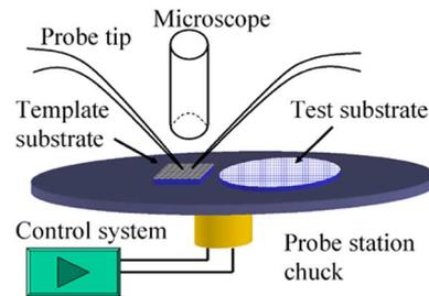
Fig. 1. Schematic of single nanowire manipulation system.
