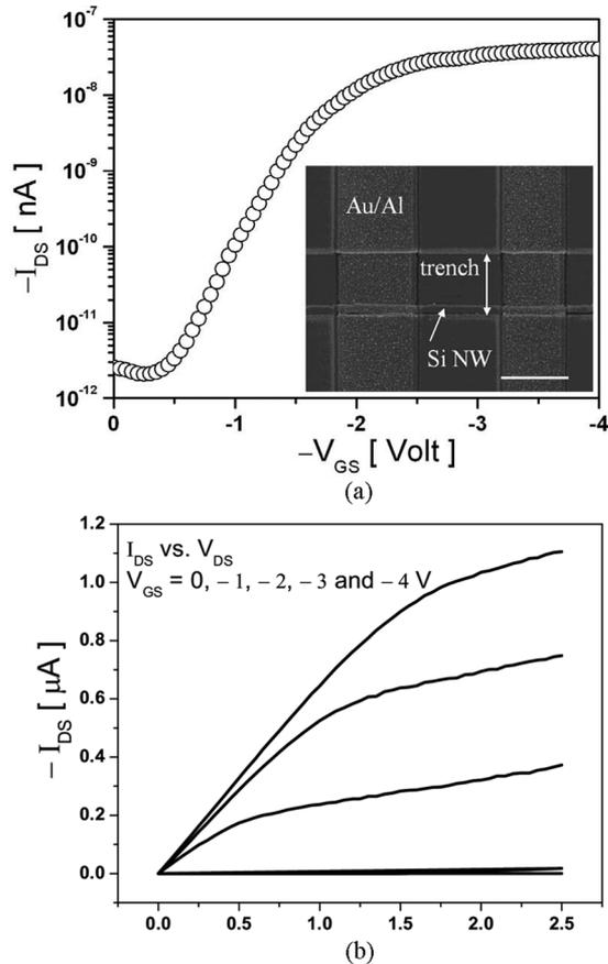
Fig. 6. (a)  $I_{DS} - V_{GS}$  with  $V_{DS} = -100$  mV and (b)  $I_{DS} - V_{DS}$  of a simple bottom-gated SiNW (145 nm in diameter) FET. Inset of (a) is SEM image (Scale bar: 3  $\mu$ m).
