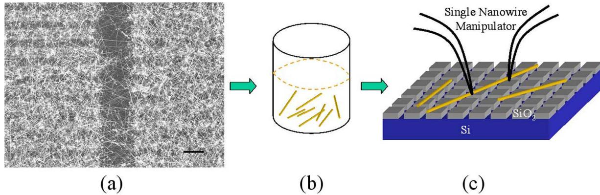
Fig. 2. (a) SEM image of Si nanowires grown from patterned Au catalyst on a silicon wafer. (b) Nanowires were removed into a suspension of DI water. A drop of the nanowire solution was dispersed on a template substrate and evaporated under a vacuum of 100 mtorr for 4 h. (c) Schematic of manipulator tips picking up a nanowire from a template substrate.
