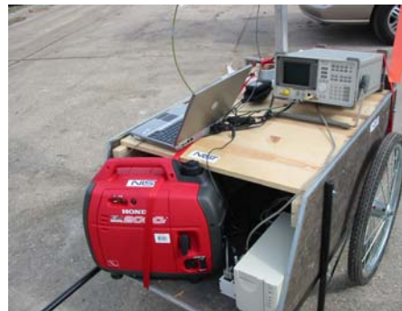
Figure 6: Measurement instruments on mobile cart.
