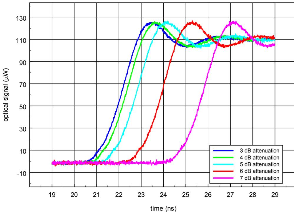
**Figure 7. Optical output of LWCM depicting delay variation as OTDR output power is varied.**
