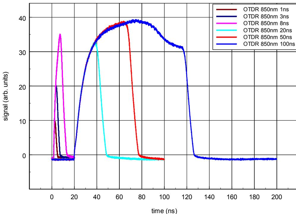
**Figure 2. OTDR output at 850 nm, available pulse widths.**
