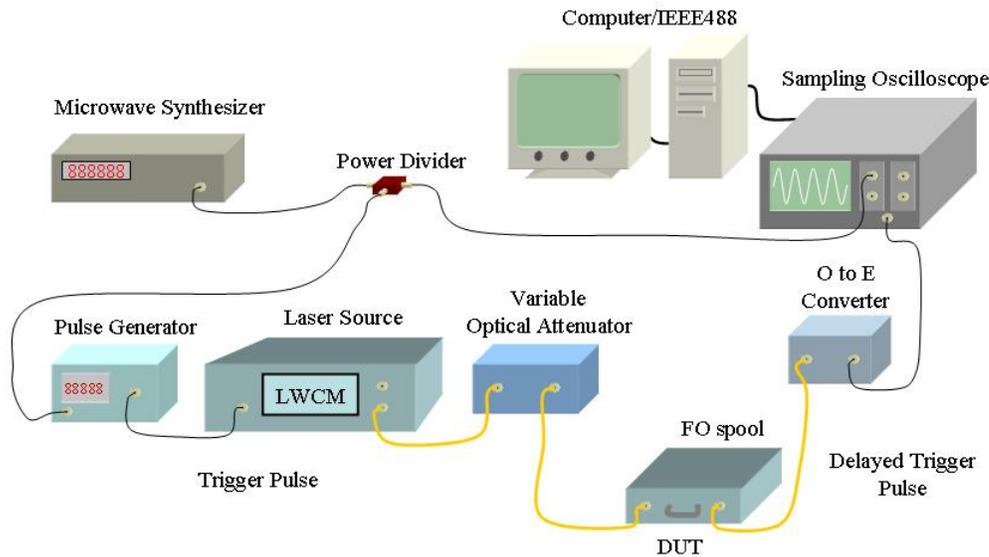
**Figure 9. Measurement system.**
