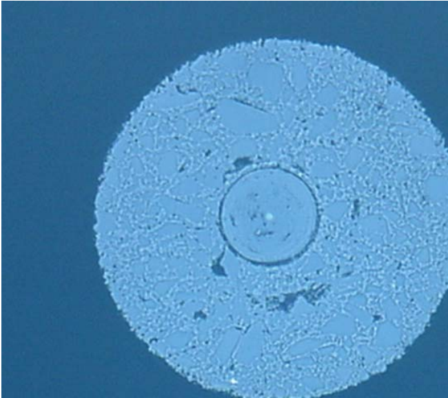
Figure 11. Magnified optical image of new, unused biconic connector.
