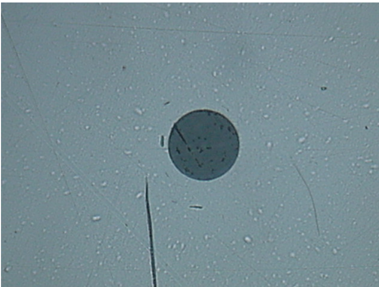
Figure 13. Magnified optical image of the same ST connector after standard cleaning. Some surface damage is visible.
