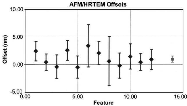
FIG. 2. Comparison of the individually estimated AFM offsets and the weighted-mean offset. The uncertainties shown in the plot are the expanded uncertainties ( $k=2$ ). The uncertainties include the reproducibility of both the HRTEM and AFM results and the influence of relative positioning uncertainty. The weighted average and expanded uncertainty ( $k=2$ ) are  $1.03 \text{ nm} \pm 0.58 \text{ nm}$ .
