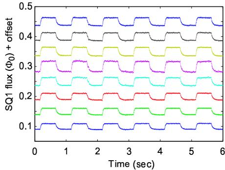
Fig. 3. Plot showing multiplexed optical response of 8 pixels to chopped narrowband  $450 \mu\text{m}$  wavelength illumination. The incident optical power on each pixel is  $1.8 \text{ fW}$ . Plots are offset for clarity.
