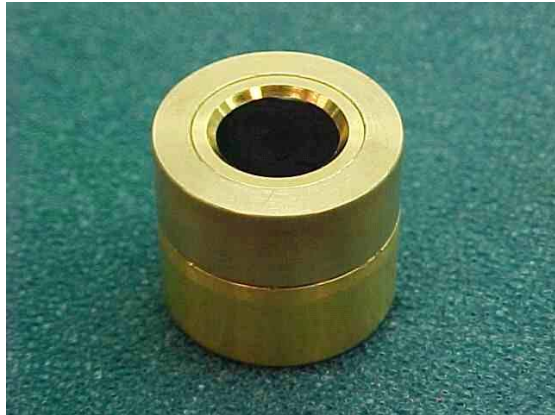
Figure 2. Photographic image of completely packaged pyroelectric detector with MWNT coating prepared by CVD.
