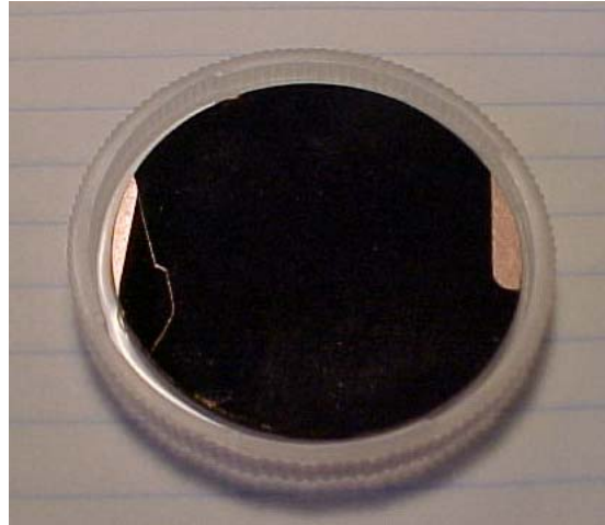
Figure 3. A photographic image of MWNTs grown on a Cu disk (the disk is 40 mm in diameter and 1 mm thick). The image shows a scratch on the left side and the absence MWNTs (non-black) where the \text{Si}_3\text{N}_4 barrier layer was absent.
