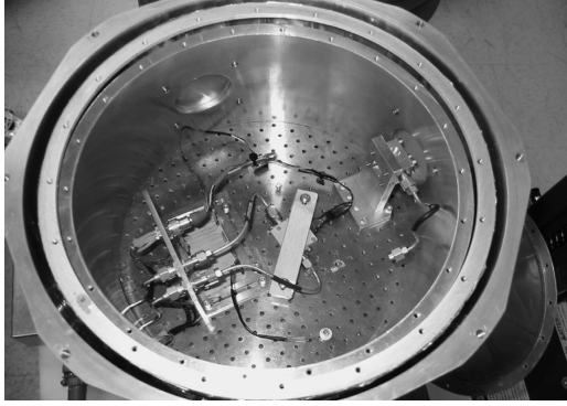
Fig. 2. Cryogenic measurement setup for the MMIC LNA. The LNA is in the center under the metal strap.
