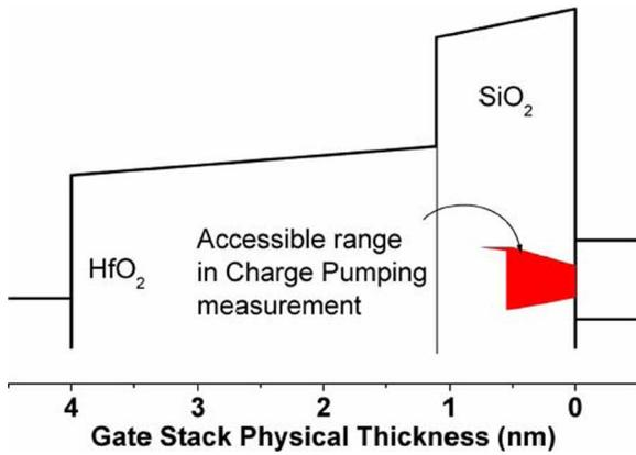
FIG. 2. Schematic of the band diagram for the high- $k$  gate stack. The CP accessible range for the employed CP measurements conditions is shown overlapping the band diagram.
