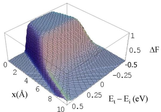
FIG. 1. 3D  $\Delta F$  contour simulation result.  $\Delta F$  is equal to one within the trapezoidal plateau, which indicates the region having the maximum probability of being probed. The parameters used in this simulation are  $t_{on/off}=50$  ns,  $t_{r/f}=30$  ns,  $V_a=1.2$  V,  $m_{e/h}=0.5/0.4$  eV,  $\Phi_{e/h}=3.1/3.8$  eV, and  $\sigma_{np}(0)=10^{-14}/10^{-16}$  cm<sup>-2</sup>.
