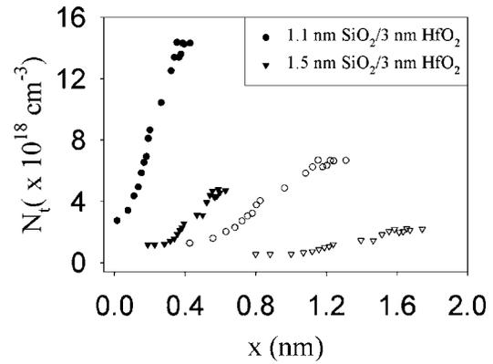
FIG. 4. The comparison of  $N_t$  in dielectrics with different thicknesses of the SiO<sub>2</sub> interfacial layer. The pure SiO<sub>2</sub>, SiO<sub>2</sub>/HfO<sub>2</sub> diffusion, and pure HfO<sub>2</sub> regions can be identified clearly in both dielectrics.
