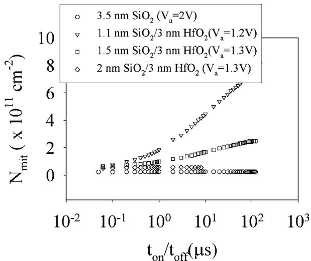
FIG. 3. The comparison of  $N_{mit}$  in dielectrics with different thicknesses of the SiO<sub>2</sub> interfacial layer. At the same depth,  $N_{mit}$  is higher for the dielectric with a thicker interfacial layer. As for the SiO<sub>2</sub> dielectric,  $N_{mit}$  is constant, which indicates no further traps exist in the bulk dielectric.
