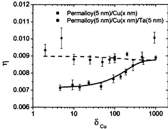
FIG. 3. Damping as a function of Cu thickness for the Permalloy (5 nm)/Cu(x nm) bilayer systems [squares, Fig. 2(b)] and a Permalloy (5 nm)/Cu(x nm)/Ta (5 nm) trilayer system (dots). The solid line represents the fit to the data using Eq. (3). The dashed line represents the fit to the data using a trilayer model with one FM/NM and one NM/NM interface (Ref. 14).
