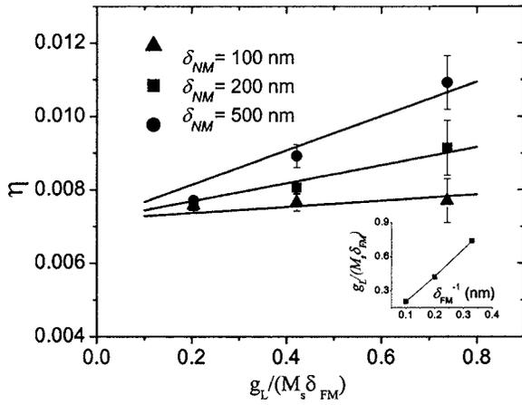
FIG. 1. Effective damping  $\eta$  as a function of three different Permalloy thicknesses  $\delta_{FM}$  and three different Cu layer thicknesses  $\delta_{NM}$ . The solid lines represent the fits from Eq. (3) for each  $\delta_{NM}$  with a fitted mixing component  $g^{1A^{-1}}=1.5 \times 10^{15} \text{ cm}^{-2}$  and a fixed diffusion length  $l_s=250 \text{ nm}$ . The inset shows the dependence of  $g_L(M_s \delta_{FM})^{-1}$  on  $\delta_{FM}^{-1}$ .
