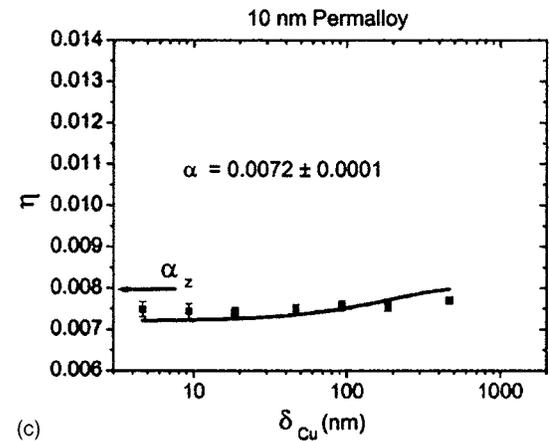
FIG. 2. Damping as a function of Cu layer thickness for three different Permalloy thicknesses: (a) 3, (b) 5, and (c) 10 nm. The solid lines represent a fit of Eq. (3) to the data using  $g^{1A^{-1}}=1.5 \times 10^{15} \text{ cm}^{-2}$  as determined by the fit in Fig. 1. The intrinsic damping  $\alpha$  and diffusion length were fitting parameters. The arrows indicate the damping of the Permalloy films without Cu cap,  $\alpha_z$ .
