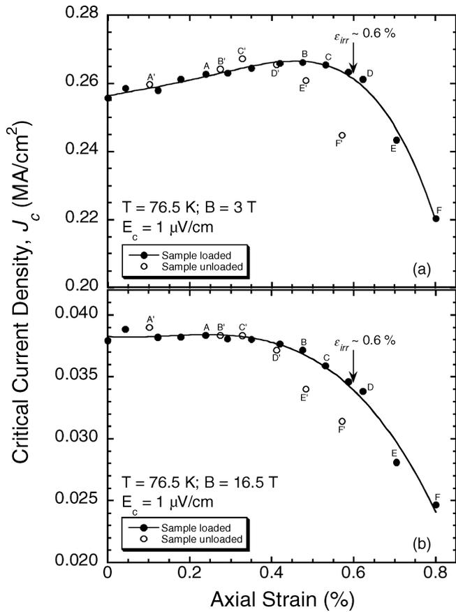
Fig. 3. Critical-current density as a function of axial tensile strain at 76.5 K for a Cu-laminated YBCO coated conductor, in magnetic fields of (a) 3 T and (b) 16.5 T, applied parallel to the YBCO (*a, b*) plane. Data when the sample was loaded and unloaded are respectively labeled by corresponding unprimed and primed letters. The irreversible strain limit  $\varepsilon_{irr}$  is about 0.6%, mostly independent of magnetic field.
