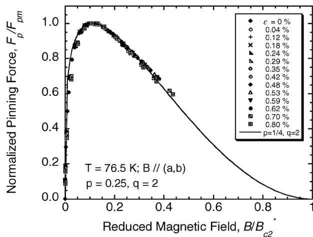
Fig. 6. Normalized pinning force density as a function of reduced magnetic field ( $b = B/B_{c2}^*$ ) at 76.5 K for a Cu-laminated YBCO coated conductor for various values of axial tensile strain up to 0.8%.  $B_{c2}^*$  is the effective upper critical field at which  $F_p(B)$  extrapolates to zero. Data show scaling of the pinning force density with reduced field for all the values of strain measured. The continuous line represents a function proportional to  $b^{0.25}(1-b)^2$ .
