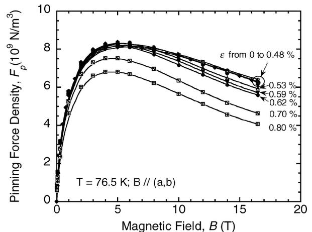
Fig. 5. Pinning force density as a function of magnetic field at 76.5 K for a Cu-laminated YBCO coated conductor for various values of axial tensile strain up to 0.8%.
