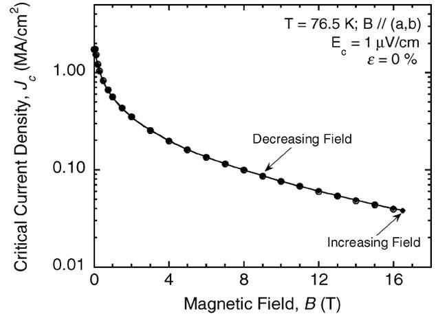
Fig. 1. Critical-current density as a function of magnetic field at 76.5 K and zero applied strain for a Cu-laminated YBCO coated conductor. Magnetic field was applied parallel to the YBCO (*a, b*) plane and perpendicular to the current-flow direction.
