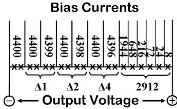
Fig. 1. High-resolution PJVS array sequence showing the number of *stacks* in each of the 13 array cells. The smallest 6 cells are divided in a trinary sequence. Pairs of the largest cells can be combined in opposition to produce the smallest voltage increments based on 1, 2, or 4 total stacks. Note that there are *twice* as many junctions as stacks for the double-junction stacks presented in this paper.
