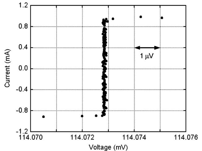
Fig. 3. High-resolution step flatness measurement showing a current range of about 2 mA measured on the 100 mV scale of a digital voltmeter. About half of the junctions (35198 JJ's) were biased on the positive voltage step and the other half (32208 JJ's) were biased on the negative voltage step, producing a smaller voltage ( $+1.342858\text{ V} - 1.228785\text{ V} = 0.114073\text{ V}$ ) that can be measured with high resolution.
