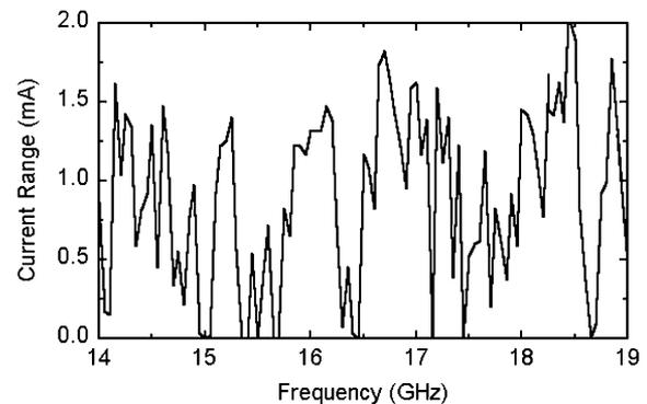
Fig. 4. Frequency dependence of the operating current range over which all junctions on the high-resolution chip produce a flat step. The power is adjusted at each frequency to maximize the current range for the entire circuit.
