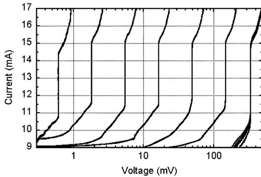
Fig. 2. Current-voltage  $IV$  characteristics for all 13 array cells from the high-resolution PJVS circuit using  $\text{MoSi}_2$  double-stacked junction arrays. All  $IV$ s were measured with the same power at 18.5 GHz. The multiple  $IV$ s with the largest voltage step correspond to the seven largest arrays with about 8800 junctions each, while the smallest step is for the cell with only 16 junctions.
