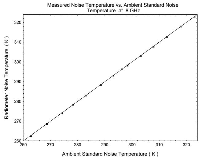
Fig. 3 Noise Measurements at 8 GHz.
