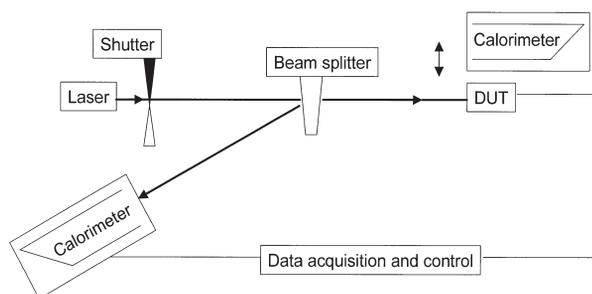
Fig. 2. Measurement scheme for C-series calorimeter measurements.
