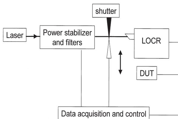
Fig. 3. Measurement scheme for the LOCR-based calibrations.
