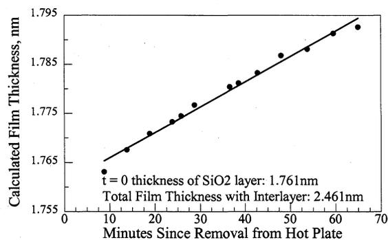
FIGURE 1. SWE results: Interface layer model - with a 0.7nm, index = 2.8 interlayer.
