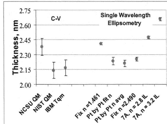
**FIGURE 7.** Thicknesses within wafer sweet Spots: Averages and standard deviations as follows - C-V (2 wafers); SWE (7 wafers).
