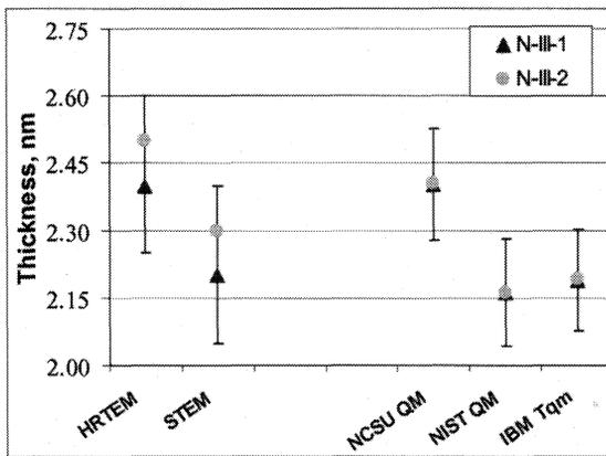
**FIGURE 6.** Thickness values and uncertainties from TEM and C-V measurements on two wafers.
