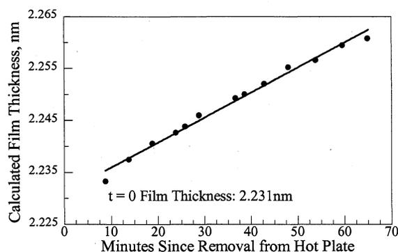
**FIGURE 3.** SWE results: Single layer model - index fixed at 2.49 - near the pt. by pt. average.
