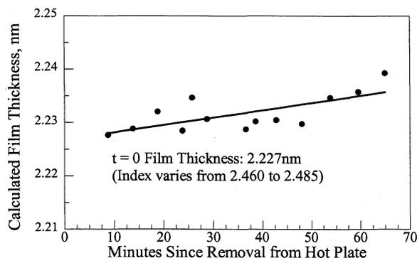
**FIGURE 2.** SWE results: Single layer model - fit on thickness and index at each point.
