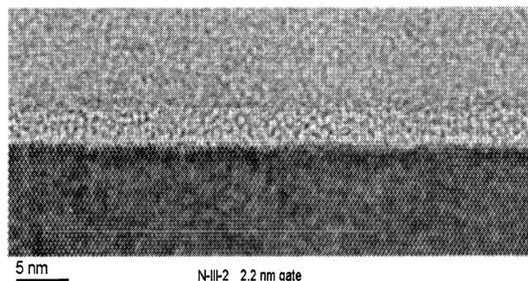
**FIGURE 4.** HRTEM image of a capacitor section on wafer N-III-2. Thin lines show the electronically generated measurement box used to determine the value of the oxide thickness (central band in photograph)
