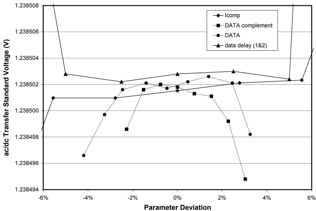
FIGURE 3. Plot showing the operating margins obtained at 8 Gbit/s using the ac/dc transfer standard and illustrating the “flat spots” for the 4 tightest parameters: amplitude (data), amplitude (data complement), data delay (both 1 & 2 moved together), and  $I_{comp}$ . One vertical division in this graph represents about 1.6 parts in  $10^6$ .
