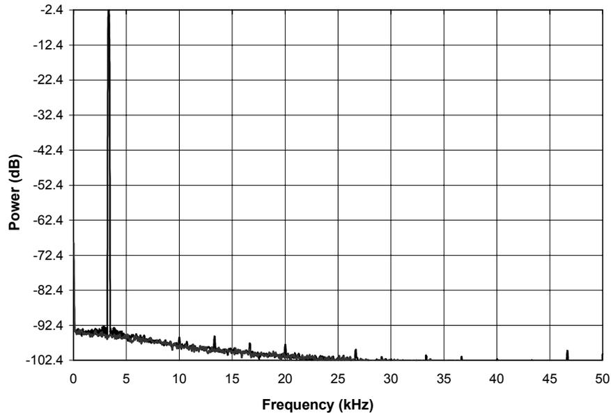
FIGURE 2. Spectrum analyzer measurement demonstrating  $-95$  dBc low distortion for the ACJVS with two Josephson arrays generating a 242 mV (zero-to-peak) sinewave at 3.3 kHz using 8200 junctions at 10 Gbit/s. The spectrum measurement used 100 Hz resolution bandwidth and 100 averages.
