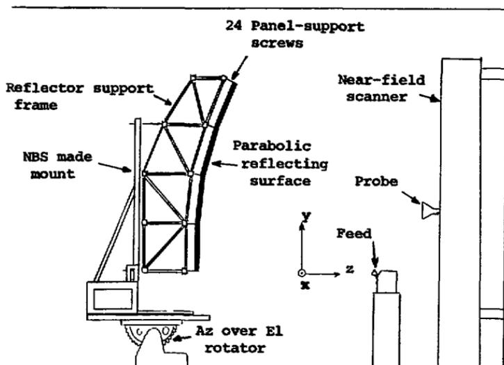
Figure 1. Measurement facility schematic and coordinate system compact range, NBS, Boulder, Colorado
