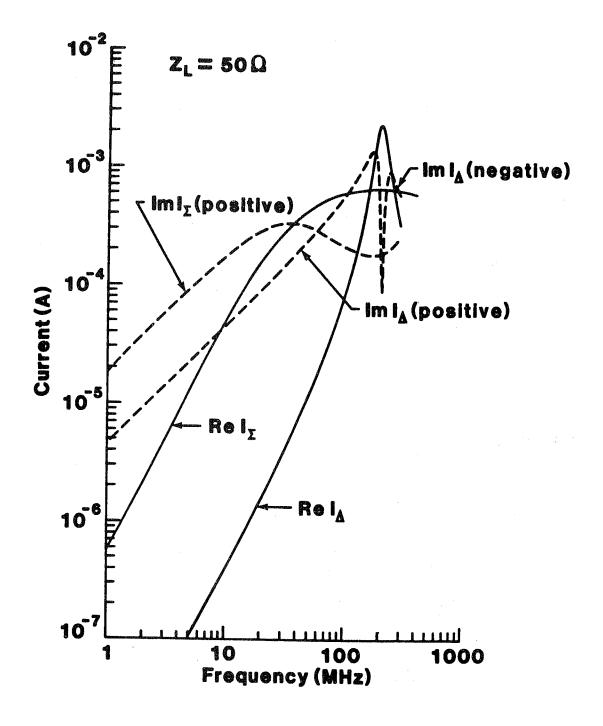
Figure 9. Magnetic-loop (I  $_{\Sigma}$ ) and electric-dipole (I  $_{\Delta}$ ) currents of loop antenna (Z  $_{L}$  = 50  $\Omega$  ).
