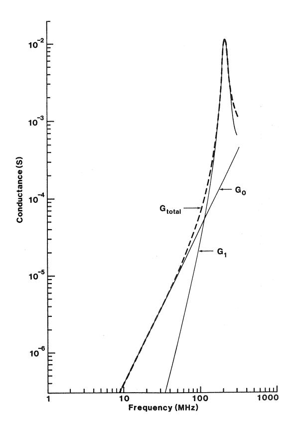
Figure 3. Conductance of loop antenna (a = 0.02 m, b = 0.16 m).
