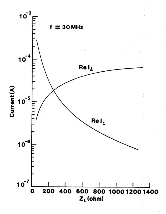
Figure 15. Real parts of magnetic-loop (I  $_{\Sigma}$ ) and electric-dipole (I  $_{\Delta}$ ) currents of loop antenna as a function of load impedance at 30 MHz.
