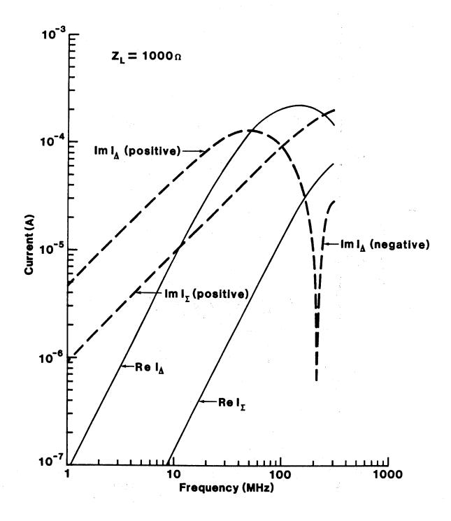
Figure 11. Magnetic-loop (I  $_{\Sigma}$ ) and electric-dipole (I  $_{\Delta}$ ) currents of loop antenna (Z  $_{L}$  = 1000  $_{\Omega}$  ).
