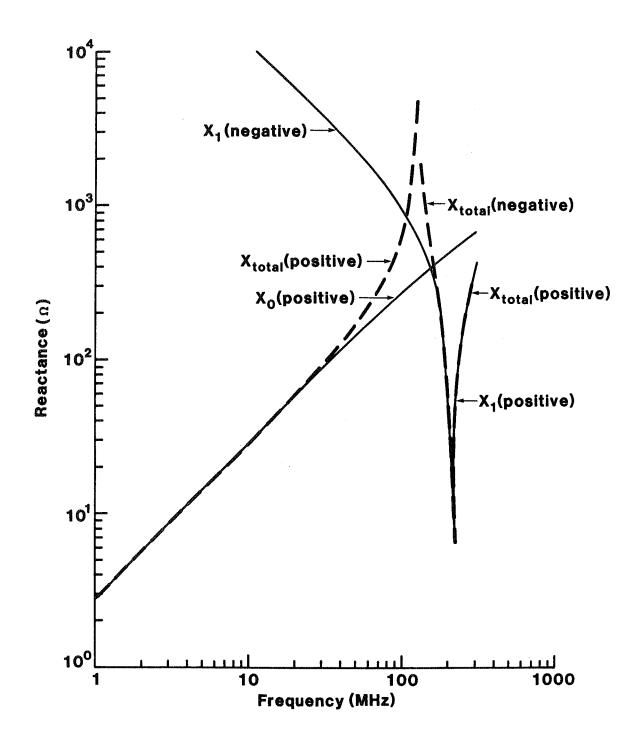
Figure 6. Reactance of loop antenna ( a = 0.02 m, b = 0.16 m).
