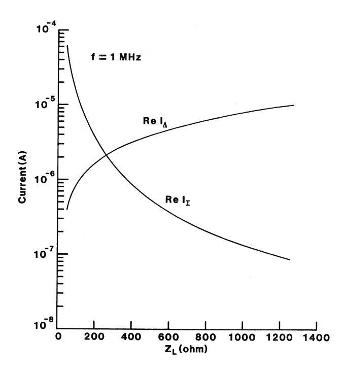
Figure 13. Real parts of magnetic-loop (I  $_{\Sigma}$ ) and electric-dipole (I  $_{\Delta}$ ) currents of loop antenna as a function of load impedance at 1 MHz.
