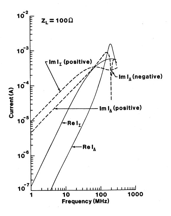
Figure 10. Magnetic-loop (I  $_{\Sigma}$ ) and electric-dipole (I  $_{\Delta}$ ) currents of loop antenna (Z  $_{L}$  = 100  $\Omega$  ).
