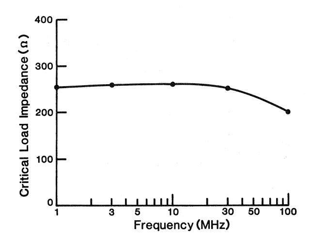
Figure 17. Critical load impedance of loop antenna as a function of frequency.
