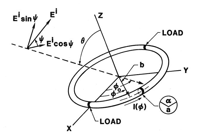
Figure 1. Loop configuration for simultaneous electric and magnetic field sensor.
