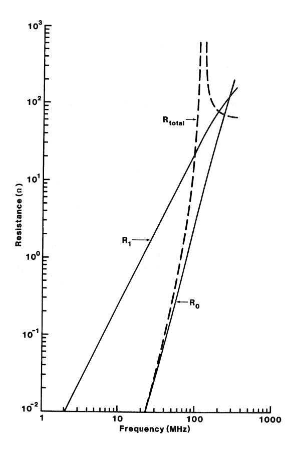
Figure 5. Resistance of loop antenna (a = 0.02 m, b = 0.16 m).
