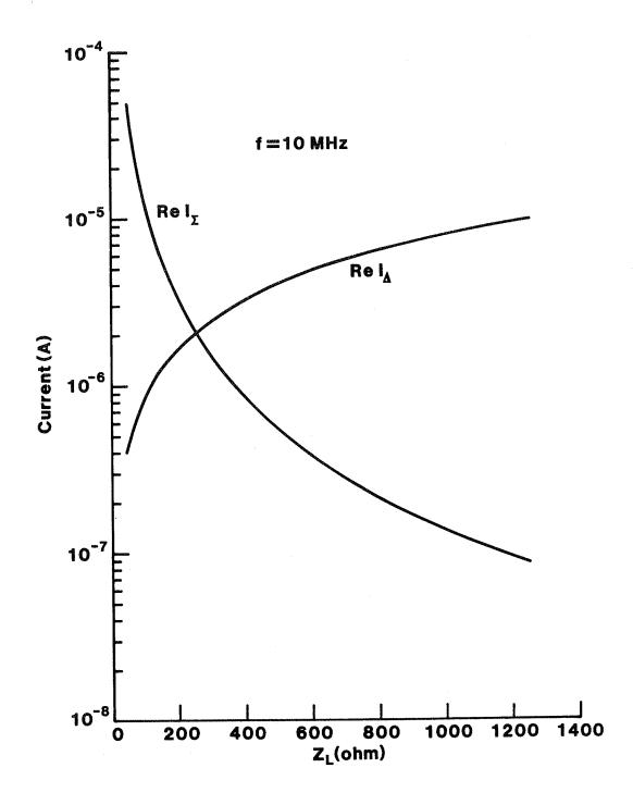
Figure 14. Real parts of magnetic-loop (I  $_{\Sigma}$ ) and electric-dipole (I  $_{\Delta}$ ) currents of loop antenna as a function of load impedance at 10 MHz.
