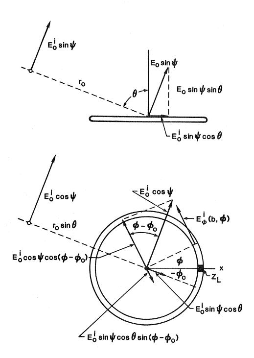
Figure 2. Receiving Loop in an incident plane-wave field.
