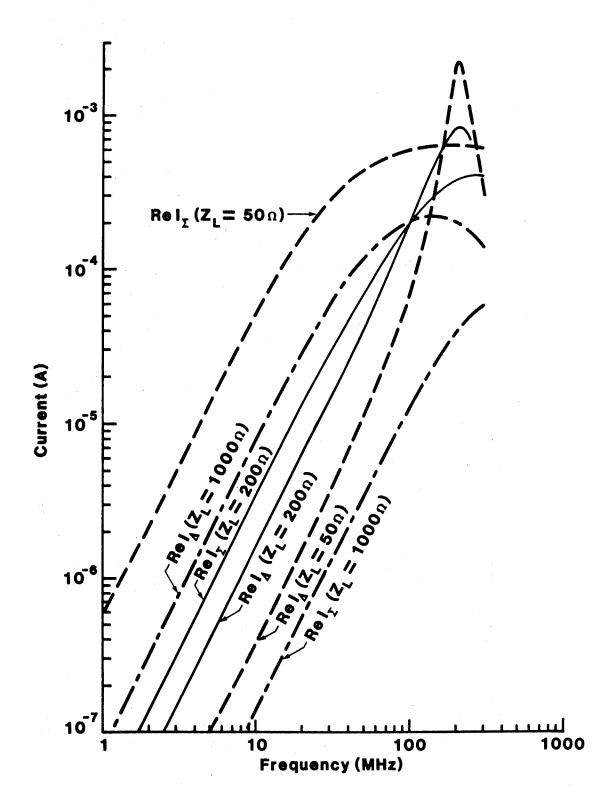
Figure 12. Real parts of magnetic-loop (I  $_{\Sigma}$  ) and electric-dipole (I  $_{\Delta}$  ) currents of loop antenna with various load impedances.
