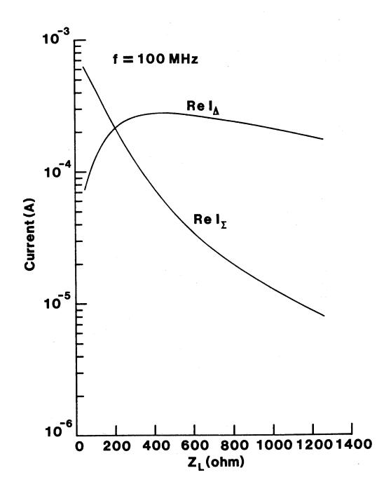
Figure 16. Real parts of magnetic-loop ( $I_{\Sigma}$ ) and electric-dipole ( $I_{\Delta}$ ) currents of loop antenna as a function of load impedance at 100 MHz.
