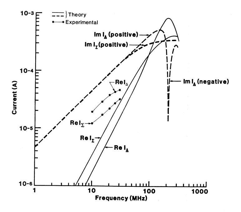
Figure 7. Magnetic-loop (I  $_{\Sigma}$ ) and electric-dipole (I  $_{\Delta}$ ) currents of loop antenna (Z  $_{L}$  = 200  $_{\Omega}$  ).
