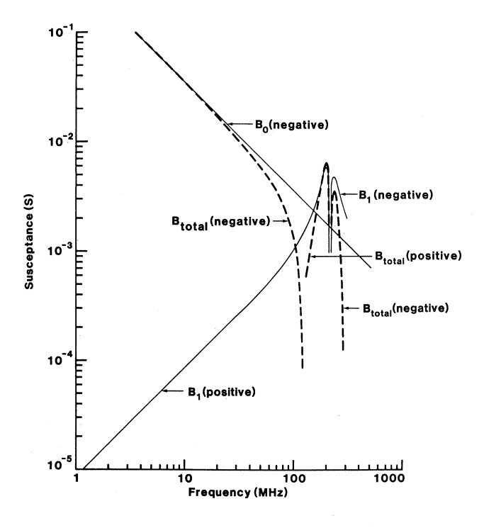
Figure 4. Susceptance of loop antenna (a = 0.02 m, b = 0.16 m).
