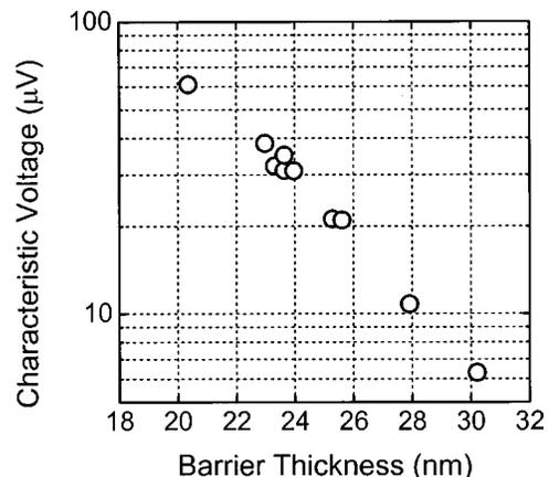
FIG. 1. Characteristic voltage ( $V_c = I_c R_n$ ) at 4 K for a range of MoSi<sub>2</sub> barrier thicknesses. The data are from arrays of single junctions and a few arrays of two- and three-junction stacks with electrode thicknesses greater than 50 nm.
