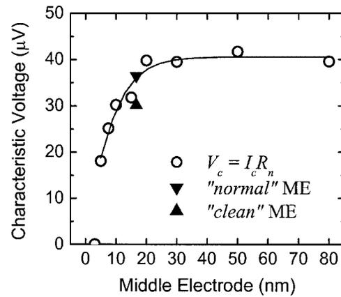
FIG. 3. Characteristic voltage  $V_c = I_c R_n$  vs middle electrode (ME) thickness  $t_{ME}$  in two-junction stacks at 4 K. At ME thicknesses of less than 20 nm, the characteristic junction voltage is suppressed. The line is drawn only as a guide for the eyes. The “normal” ME was prepared with the usual process, and the “clean” ME was prepared immediately after depositing 10 Nb films in sequence.
