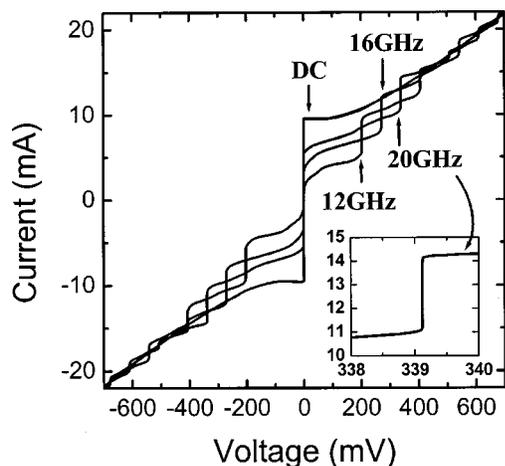
FIG. 4. Current–voltage characteristics of a 4100-stack double-barrier array (8200 series junctions) with 20 nm ME thickness biased at different microwave frequencies. These curves are qualitatively the same as those of thicker ME samples. The inset shows the  $n=1$  Shapiro step with  $\sim 3$  mA step height with a 20 GHz microwave bias.
