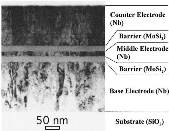
FIG. 2. Cross-sectional TEM image of a five layer Nb/(MoSi<sub>2</sub>/Nb)<sub>2</sub> film. Each of the barriers is 23 nm thick and the middle electrode thickness is 20 nm.
