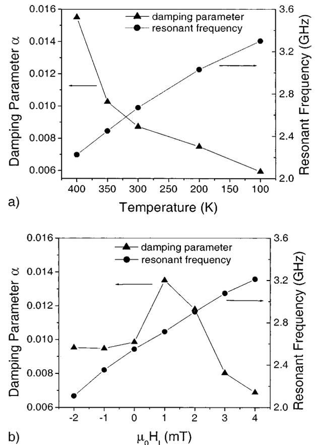
FIG. 4. The resonant frequencies and damping parameters determined from fitting the noise data for (a) the temperature-dependent data with no applied longitudinal field, and for (b) the longitudinal field dependent data at 300 K.
