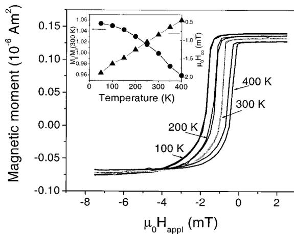
FIG. 3. Magnetic moment as a function of applied field for a coupon from the spin valve wafer. The field was applied parallel to the fixed-layer magnetization. The hysteresis loops are not centered around zero moment because of the fixed moment of the pinned layer. The inset shows the measured coupling field and relative free layer saturation magnetization calculated from the hysteresis loops.
