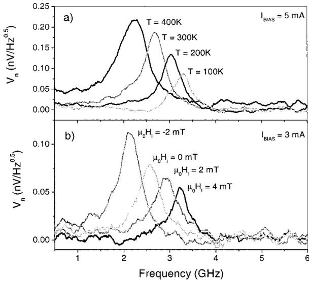
FIG. 1. Voltage noise spectra of a  $1 \mu\text{m} \times 3 \mu\text{m}$  spin valve device for (a) a series of substrate temperatures with no applied longitudinal field, and (b) a series of longitudinal bias fields at room temperature. Both sets of curves are similar, with the resonant frequency increasing and the noise amplitude decreasing as the stiffness fields increase.
